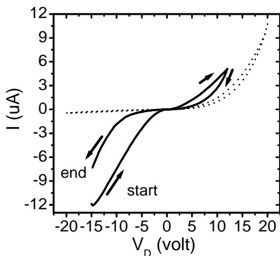
Fig. 2. Currents measured before (solid line) and after (dashed line) 7 days of air exposure. The voltage at L changes, while U is kept at 0 V. Air exposure decreased currents on negative side, because electron current is blocked by oxygen doping.
