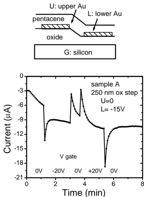
Fig. 1. Schematic diagram of the device structure, and time dependence of drain current (channel width 500  $\mu\text{m}$ ). The contacts are denoted as U (upper contact), L (lower contact), and G (gate). Current was measured with  $G = 0 \text{ V}$ ,  $U = 0 \text{ V}$ , and  $L = -15 \text{ V}$ .
