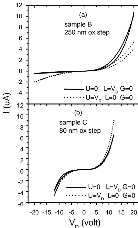
Fig. 3. Effect of oxide height on drain currents. Currents were measured after 7 days of air exposure. Voltage at U is zero in solid lines, and voltage at L is zero in dashed lines. (a) When the oxide step is high (250 nm), electric field strength at L is much stronger than the field at U. On negative voltage side, electron injection at L is blocked. (b) When the oxide step is small (80 nm), electric fields at L and U are almost same, and current shows symmetric behavior.
