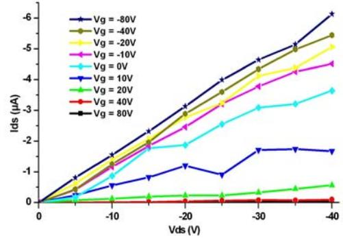
Fig. 3 Output characteristics measured on one of the fabricated PMOS-like CNTFET structures.
