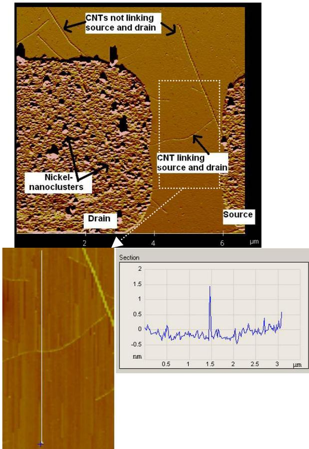
Fig. 2 AFM (tapping-mode) amplitude image of a structure (top), topography image of the linking CNT (bottom left) and cross-section along the white line (bottom right).
