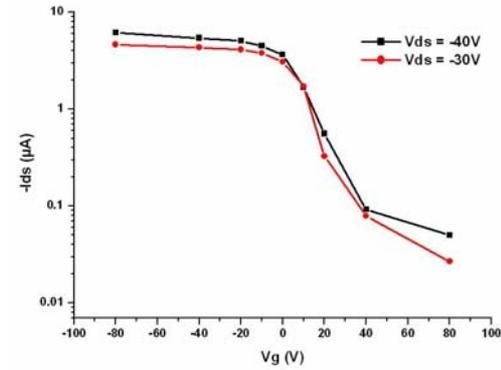
Fig. 4 Sub-threshold voltage characteristics of CNTFET (same device as fig. 3).
