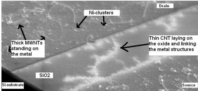
Fig. 1 SEM image of a test structure. (The wafer has been cut and tilted). The thin CNTs are visible on the oxide only because of charging effects.
