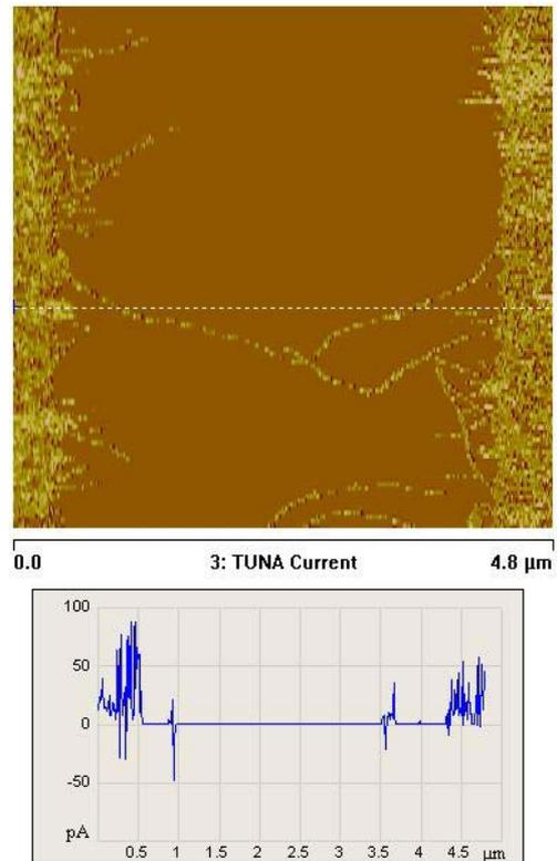
Fig. 5 Conductive AFM current image (top) and cross-section along the white line (bottom). Bias applied to the chuck: -20 mV.
