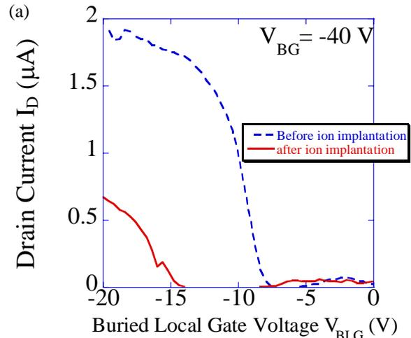
Fig. 2 (a),  $I_D - V_{BLG}$  characteristics at  $V_{BG} = -40V$  before and after oxygen ion implantation.
