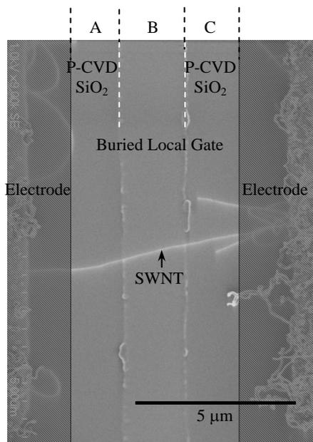
Fig. 1 (b), Top view of SWNT-FET with BLG by SEM observation.
