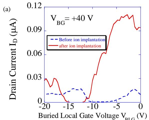
Fig. 3 (a),  $I_D - V_{BLG}$  characteristics at  $V_{BG} = 40V$  before and after oxygen ion implantation
