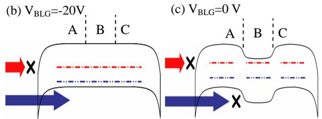
Fig. 2 (b), (c), Schematic band diagram of SWNT-FET with BLG (b) at  $V_{BLG} = -20V$ , (c) at  $V_{BLG} = 0V$ . The line - · - · - indicates the Fermi level before (after) ion implantation.
