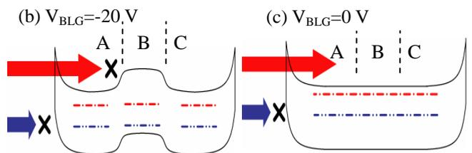
Fig. 3 (b), (c), Schematic band diagram of SWNT-FET with BLG (b) at  $V_{BLG} = -20V$ , (c) at  $V_{BLG} = 0V$ . The line - · - · - indicates the Fermi level before (after) ion implantation.
