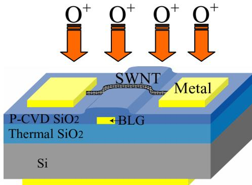
Fig. 1 (a), Schematic sample structure of SWNT-FET with BLG and back gate.
