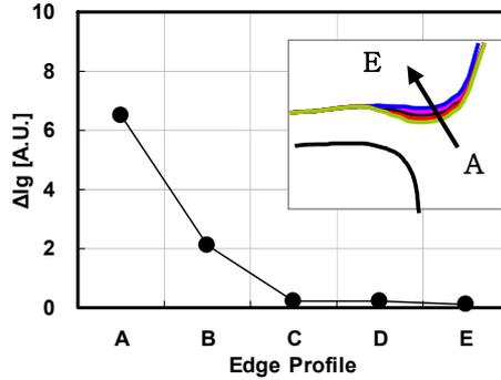
**Fig. 7.** Simulated F-N Tunneling current in SAP process active profile.
