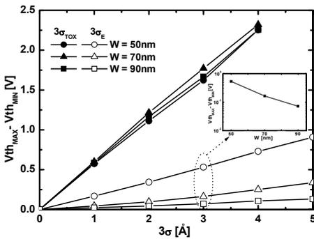
**Fig. 9.** Simulated  $V_{th}$  dispersion vs. process random variation for different cell widths in SAP
