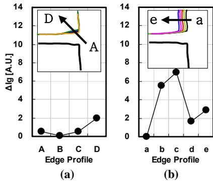
**Fig. 6.** Simulated F-N tunneling current in SA-STI process active profile.
