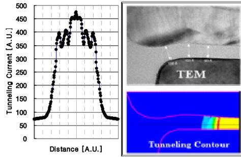
**Fig. 4.** SAP process active profile and F-N tunneling simulation for erase.
