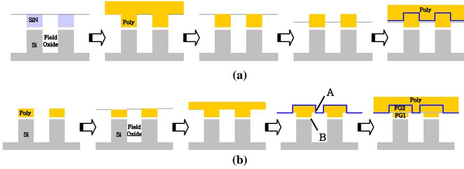
**Fig. 1.** Process sequence. (a) SAP (Self-Aligned Poly) Process (b) SA (Self-Aligned)-STI Process
