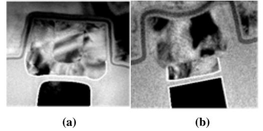
**Fig. 2.** TEM cross section of (a) SAP process cell and (b) SA-STI process cell
