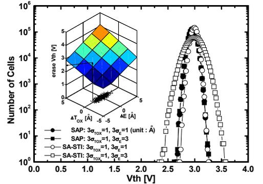
**Fig. 8.** Simulated erase  $V_{th}$  dispersion with process random variations ( $3\sigma_{TOX}$  &  $3\sigma_E$ ) in SAP and SA-STI
