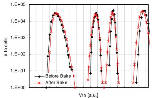
**Fig. 11.** Multi-level  $V_{th}$  distribution of SAP process cell. The retention characteristics before and after high temperature bake, 24 hours at  $150^\circ\text{C}$  after 10k cycling
