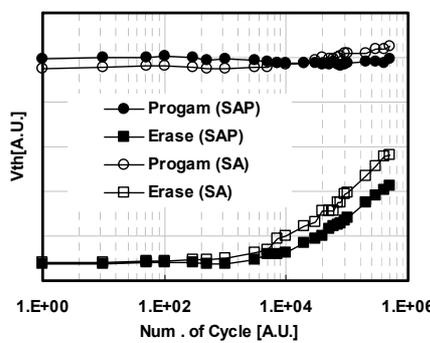
**Fig. 10.** Endurance characteristics of SAP and SA-STI process cells.
