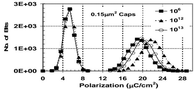
Fig. 7 Bit distribution measurements through  $10^{13}$  cycles at 1.5V.
