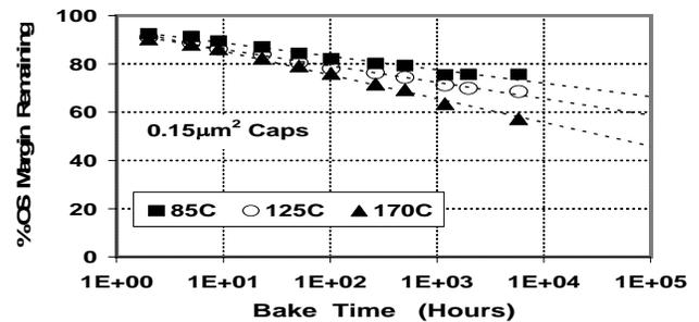
Fig. 8 Opposite state margin remaining plotted against bake temperature and time for packaged  $0.15\mu\text{m}^2$  memory cap arrays.
