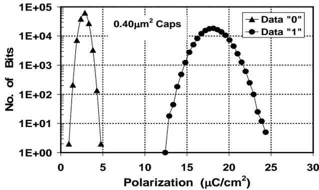
Fig. 2 Bit distribution histogram taken at 1.5V for 144kb segment. Good separation and sense margin are evident.
