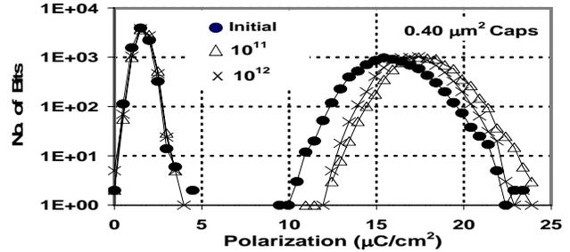
Fig. 5 Bit distribution measurements through  $10^{12}$  cycles at 1.5V.
