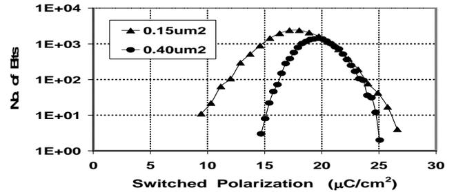
Fig. 6 Bit distribution histogram taken at 1.5V for two cap sizes.
