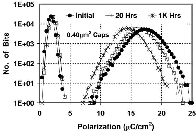
Fig. 3 Opposite State bit distribution plotted as a function of cumulative bake time. Opposite State Read 1 controls the magnitude of signal margin remaining.
