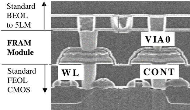
Fig. 1 Cross-sectional scanning electron micrograph illustrating placement of the FRAM module between CONT and MET1 levels.
