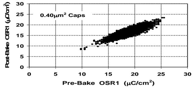
Fig. 4 Plot of post-bake OSR1 (150°C for 1000hrs) against pre-bake OSR1, expressed in polarization, for  $0.40\mu\text{m}^2$  caps.
