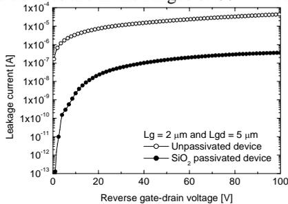
Fig. 4. Measured leakage current of the AlGaIn/GaN HFET
