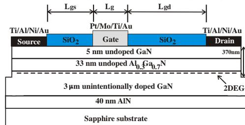
Fig. 1. Cross-sectional view of ICP-CVD SiO<sub>2</sub> passivated AlGaN/GaN HFET.
