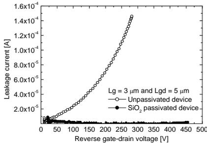
Fig. 5. Measured breakdown voltage of the AlGaIn/GaN HFET
