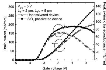
Fig. 2. Measured transfer characteristics of the AlGaN/GaN HFET
