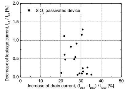
Fig. 6. Passivation effects for several AlGaIn/GaN HFETs.
