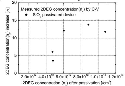
Fig. 7. 2DEG changes of the several AlGaIn/GaN HFETs after passivation
