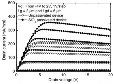
Fig. 3. Measured current-voltage characteristics of the AlGaIn/GaN HFET
