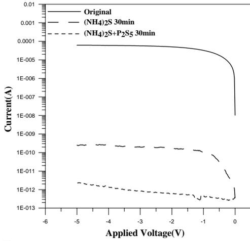
Fig.1 The I-V curves of Schottky diodes treated by original (no sulfur treatment),  $(\text{NH}_4)_2\text{S}_x$  and  $\text{P}_2\text{S}_5/(\text{NH}_4)_2\text{S}_x$ , respectively.
