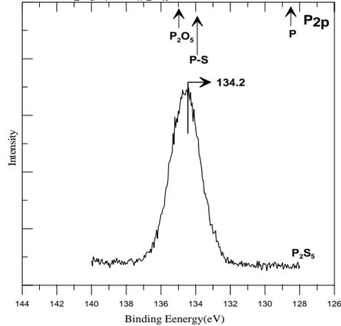
Fig.5 The P(2p) XPS spectra of samples by the  $(\text{NH}_4)_2\text{S}_x$  and the  $\text{P}_2\text{S}_5/(\text{NH}_4)_2\text{S}_x$  treatment.
