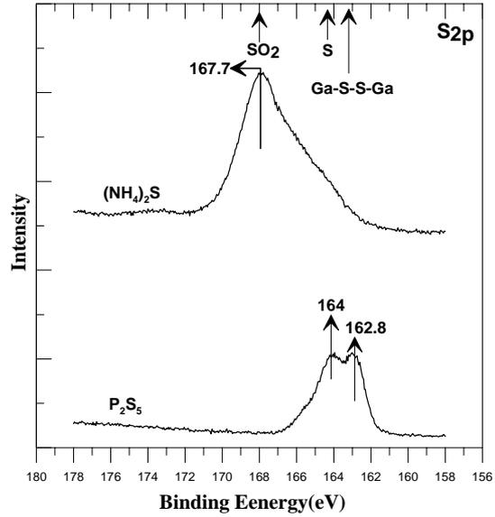
Fig.4 The S(2p) XPS spectra of samples by the  $(\text{NH}_4)_2\text{S}_x$  and the  $\text{P}_2\text{S}_5/(\text{NH}_4)_2\text{S}_x$  treatment.
