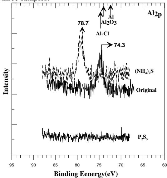
Fig.3 The correspondent Al(2p) XPS spectra measured from those three samples.
