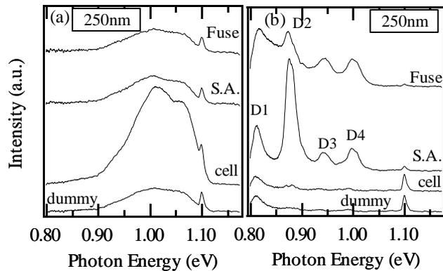
Fig. 3 CL spectra of the samples with the SiN thickness of 250nm (a) after the trench patterning and (b) after the liner oxidation.
