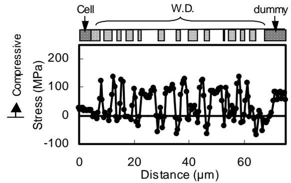
Fig. 4 Stress distribution of the sample with the SiN thickness of 250nm after the trench patterning.
