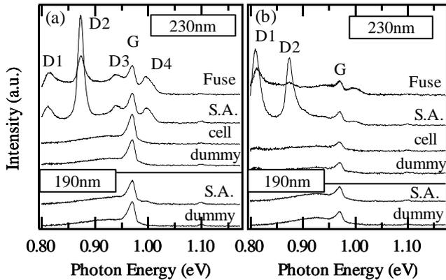
Fig. 2 CL spectra of the samples with different SiN film thickness (a) after the CMP and (b) after the sacrificial oxidation.
