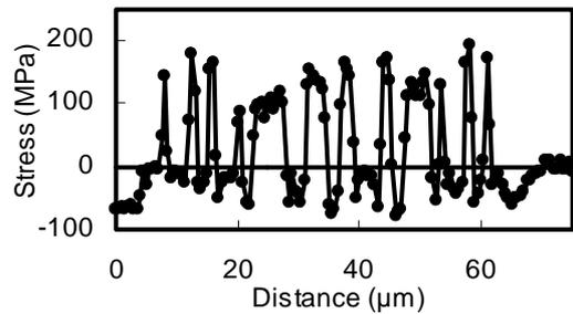
Fig. 5 Stress distribution of the sample with the SiN thickness of 250nm after the liner oxidation.
