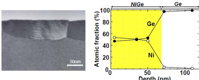
Fig. 2 Cross-sectional TEM image of nickel-monogermanide / Ge heterostructure and its EDX depth profile.
