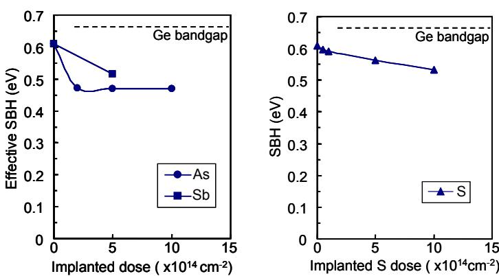
Fig. 6 Effective SBH as a function of implanted As or Sb dose.
