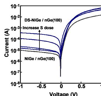
Fig. 7 I-V characteristics of NiGe/Ge (100) Schottky diodes with and without S implantation.
