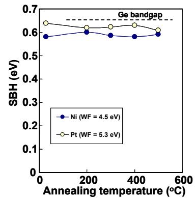
Fig. 3 Annealing temperature dependence of SBH for Nickel germanide / Ge(100) and platinum germanide / Ge(100).
