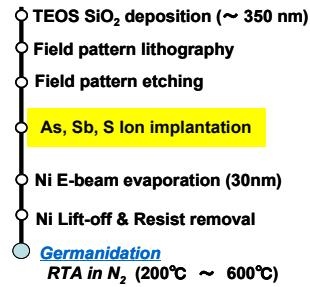
Fig. 1 Fabrication process flow of NiGe / Ge Schottky diodes.
