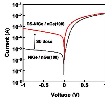
Fig. 5 I-V characteristics of NiGe/Ge (100) Schottky diodes with and without Sb implantation.
