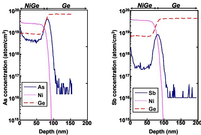
Fig. 4 Backside SIMS profiles of a) As and b) Sb dopant segregation in NiGe/Ge Schottky diodes. Implanted dose was  $5 \times 10^{15} \text{ cm}^{-2}$ . Deposited Ni thickness was 30nm.
