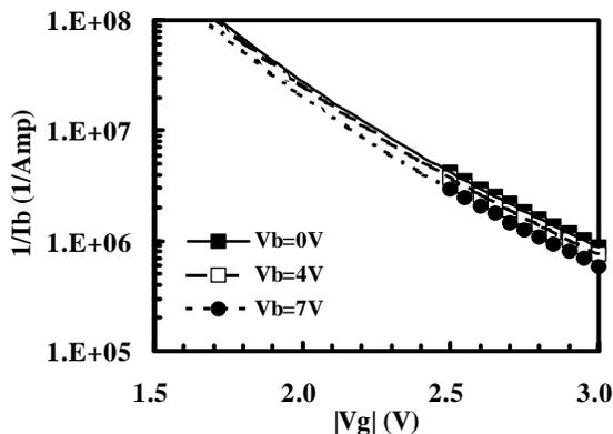
Fig. 3  $1/I_b$  versus gate bias with  $V_b=0V$ , 4V, and 7V
