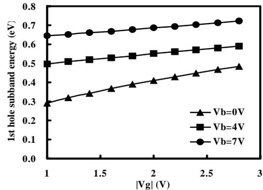
Fig. 5 Simulation of 1<sup>st</sup> subband channel hole energy at various  $V_g$  with  $V_b=0V$ , 4V, and 7V.
