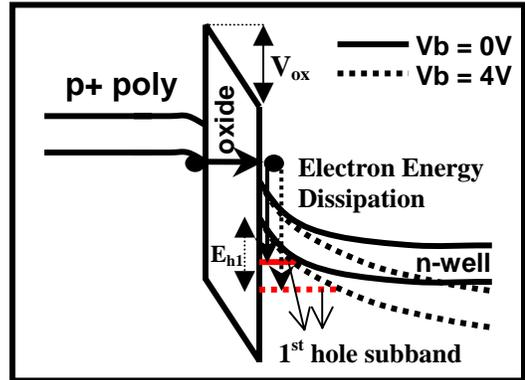
Fig. 4 Illustration of band diagram showing the electron dissipation energy at the anode interface with/without a reverse substrate bias. The electrons dissipate more energy when  $V_b=4V$ .
