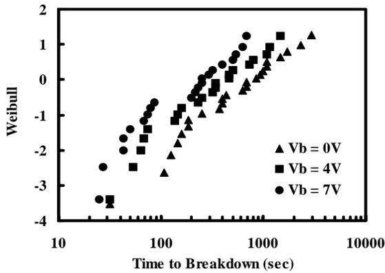
Fig. 1 Weibull distribution of time to breakdown (TBD) on pMOSFETs. The stress gate bias is -2.9V with  $V_b=0V$ , 4V, and 7V respectively.
