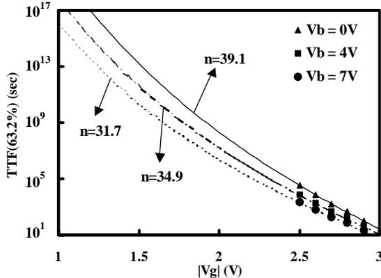
Fig. 2 Stress gate bias dependence of TDDB lifetime. The symbols are experimental data and the curves are extrapolated by the power law model.
