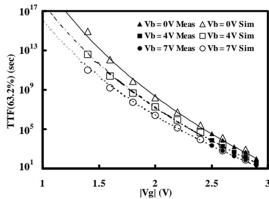
Fig. 6 Lifetime versus  $V_g$  plot of measurement and simulation data with various substrate biases.
