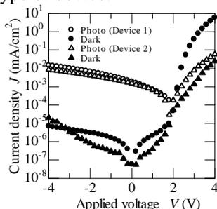
Fig.5 Current density versus voltage of OPD.
