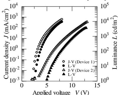
Fig.4 Luminance/current density versus voltage characteristics of OLED.
