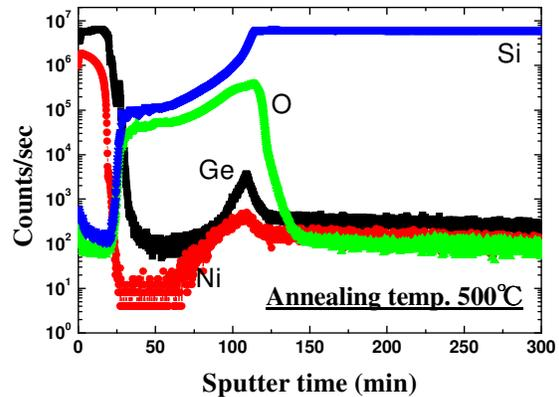
Fig. 7 SIMS profiles of NiGe/SiO<sub>2</sub>/Si substrate structure formed by nickel germanidation of GOI.
