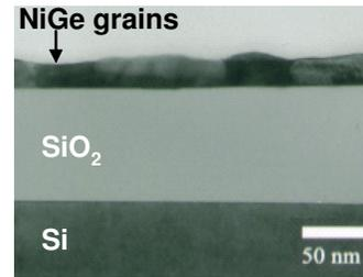
Fig. 5 TEM image of NiGe film with an initial nickel thickness of 20 nm.
