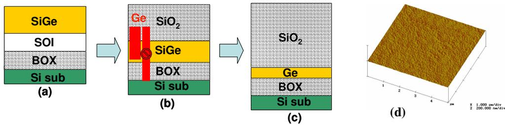
Fig.1. Process sequence for germanium condensation (a) ~ (c) and AFM image of GOI layer formed by germanium condensation (RMS=0.84nm) (d).
