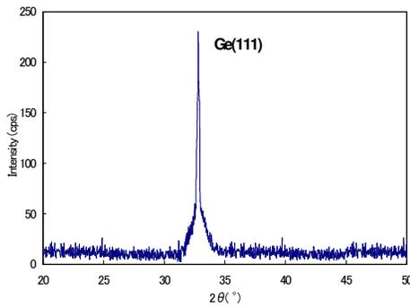
Fig.2 XRD pattern of GOI layer formed by Ge condensation.
