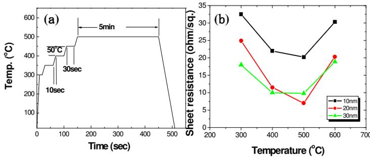
Fig. 4 Temperature history(a) and sheet resistance of nickel germanide as a function of annealing temperature(b).
