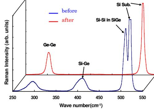
Fig.3 Raman spectra of GOI layer formed by Ge condensation.
