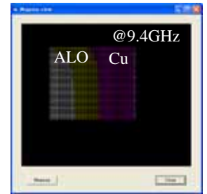
Fig.8 Reflection intensity mapping of \text{Al}_2\text{O}_3/\text{Cu} -plate.
