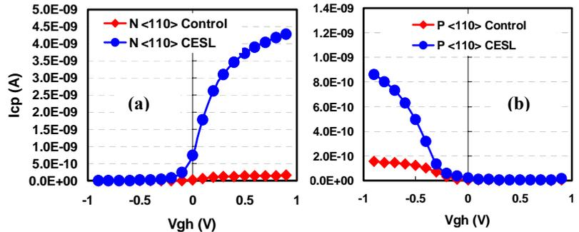
Fig. 8 High tensile stress CESL induced higher charge pumping current on both (a) NMOS and (b) PMOS.
