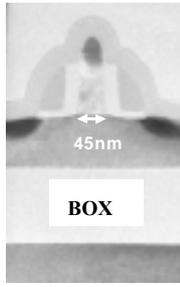
Fig. 1 Cross-sectional TEM view of SOI wafer with 45 nm channel length.
