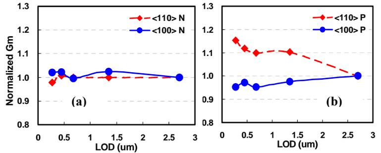
Fig. 9 (a) NMOS, (b) PMOS LOD mobility trend of  $\langle 110 \rangle / (100)$  and  $\langle 100 \rangle / (100)$  orientated SOI wafers.
