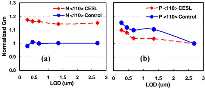
Fig. 4 The LOD mobility trend of high and low tensile stress CESL on  $\langle 110 \rangle / (100)$  SOI wafer, (a) NMOS, (b) PMOS.
