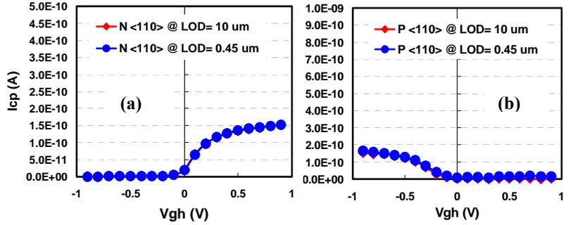
Fig. 7 (a) NMOS, (b) PMOS charge pumping current stays the same while changing LOD dimension on  $\langle 110 \rangle / (100)$  orientated SOI wafers.
