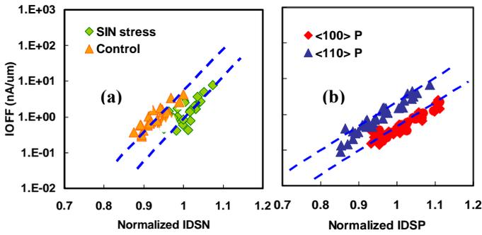
Fig. 3 Mobility enhancement approaches demonstrated 8% and 10% current gain by (a) high tensile stress CESL (b)  $\langle 100 \rangle / (100)$  wafer on N/PMOS, respectively.
