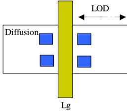
Fig. 2 Test key design of LOD effect, with various LOD dimensions.
