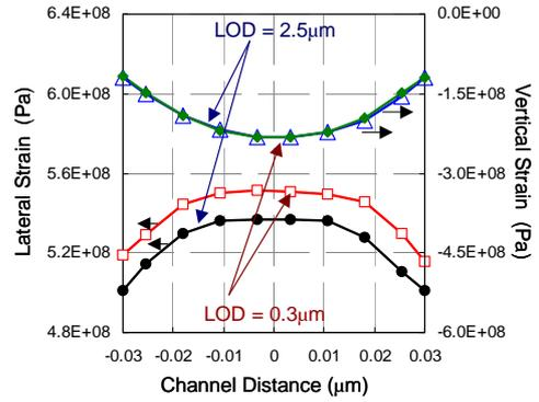
Fig. 6 Simulation data of CESL induced channel stress on LOD = 2.5 um and 0.3 um, STI stress was assumed to be negligible in this simulation.
