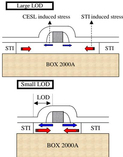
Fig. 5 Schematic of channel region stress induced by CESL and STI. Channel tensile stress induced by CESL stress is amplified when LOD size is reduced.
