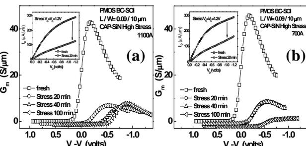
Fig. 14.  $G_m$  characteristics of 90nm BC-SOI pMOSFET with (a) 1100A (b) 700A high stress GC liner-SiN after 100 min hot carrier stressing. The insert shows the  $I_D$ - $V_D$  characteristics. Both devices show unstable characteristics during hot-carrier stressing process.
