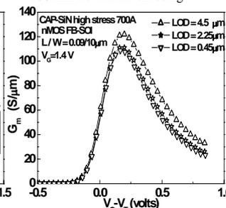
Fig. 11.  $G_m$  of 90nm FB-SOI nMOSFETs with various LOD.
