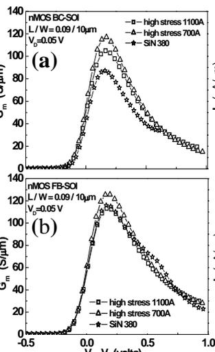
Fig. 6.  $G_m$  of 90nm (a)BC-SOI (b)FB-SOI nMOSFETs with various stress GC liner-SiN thicknesses.
