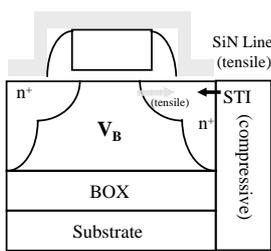
Fig. 1. The stress item in MOSFET channel region. High stress liner-SiN induces a tensile stress, and STI induces a compressive one.
