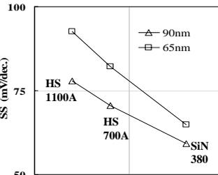
Fig. 3. Subthreshold Swing of BC-SOI nMOSFETs with various stress GC liner-SiN layers.
