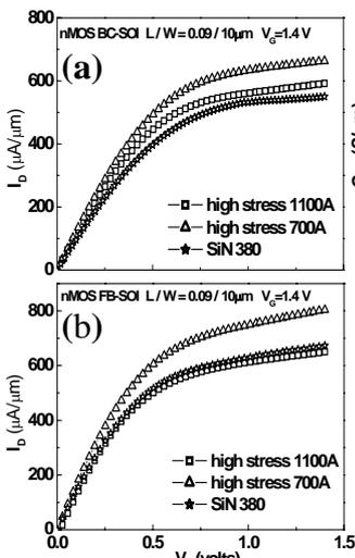
Fig. 5.  $I_D$ - $V_D$  of 90nm (a)BC-SOI (b)FB-SOI nMOSFETs with various stress GC liner-SiN thicknesses.
