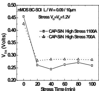
Fig. 9.  $V_{TH}$  variation of 90nm BC-SOI nMOSFET with different high stress GC liner-SiN after 100 min hot carrier stressing.
