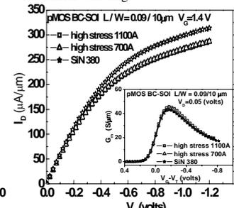
Fig. 12.  $I_D$ - $V_D$  of 90nm BC-SOI pMOSFETs with various stress GC liner-SiN thicknesses. The insert shows the  $G_m$  characteristics.
