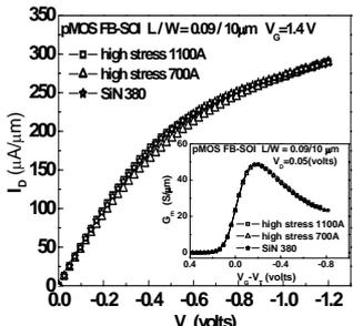
Fig. 13.  $I_D$ - $V_D$  of 90nm FB-SOI pMOSFETs with various stress GC liner-SiN thicknesses. The insert shows the  $G_m$  characteristics.
