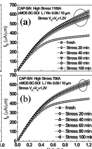
Fig. 7.  $I_D$ - $V_D$  of 90nm BC-SOI nMOSFET with (a) 1100A (b) 700A high stress GC liner-SiN after 100 min hot carrier stressing.
