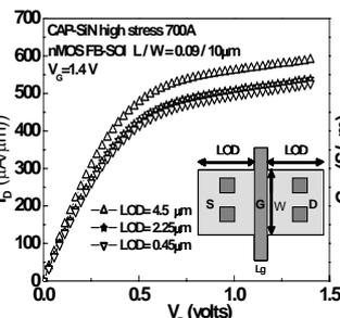
Fig. 10.  $I_D$ - $V_D$  of 90nm FB-SOI nMOSFETs with various LOD. The insert shows the design of LOD.
