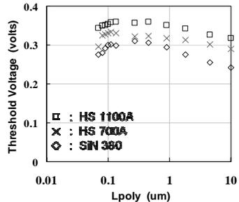
Fig. 2.  $V_{TH}$  of BC-SOI nMOSFETs with various stress GC liner-SiN layer.
