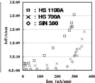
Fig. 4.  $I_{ON}$ - $I_{OFF}$  characteristics of BC-SOI nMOSFETs with various stress GC liner-SiN layer.
