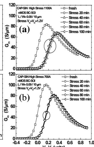
Fig. 8.  $G_m$  of 90nm BC-SOI nMOSFET with (a) 1100A (b) 700A high stress GC liner-SiN after 100 min hot carrier stressing.
