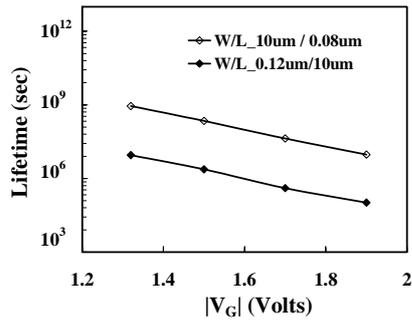
Fig. 2 Geometry dependence evaluation on NBTI.
