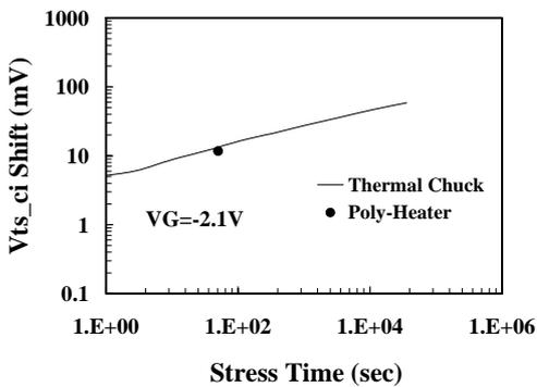
Fig. 9 Consistency check of NBTI degradation by using chuck and embedded-poly heater.
