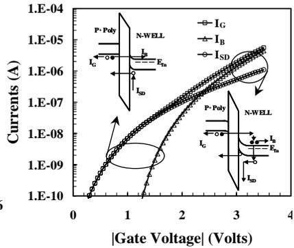
Fig. 10 Measured terminal currents of charge separate bias configuration. The energy band diagrams depict NBTI and TDDB regimes respectively.
