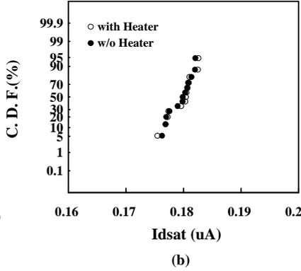
Fig. 4 Measured (a) threshold voltages, and (b) saturation currents of PMOSFETs with and without poly-heater.
