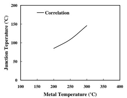
Fig. 8 Correlation plot of junction temperature and metal temperature.
