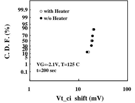
Fig. 5 Conventional NBTI test on PMOSFETs with and without poly-heater.
