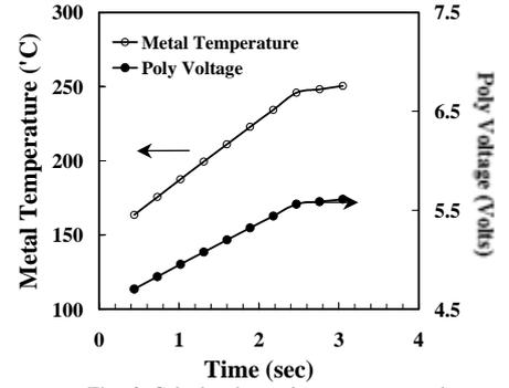
Fig. 3 Calculated metal temperature and measured poly voltage during ramp up procedure.
