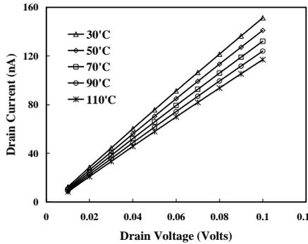
Fig. 6 Measured drain terminal currents under different ambient temperatures.
