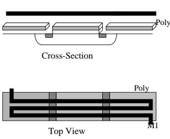
Fig. 1 Cross section view and top view of embedded poly-heater PMOSFET.
