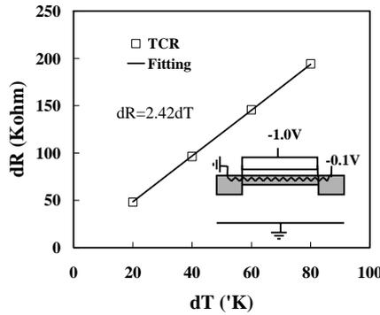
Fig. 7 Calculated turn-on resistances under different ambient temperatures.
