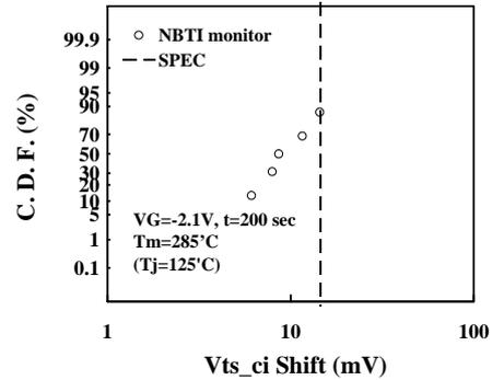
Fig. 11 A real case in-line NBTI monitor on 90nm CMOS technology.
