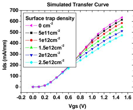
Fig. 1 Simulated transfer curves of E-pHEMT for various trap density of side recess region
