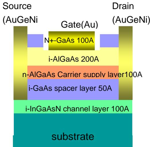
Fig. 1 The structure of InGaAsN HEMT.
