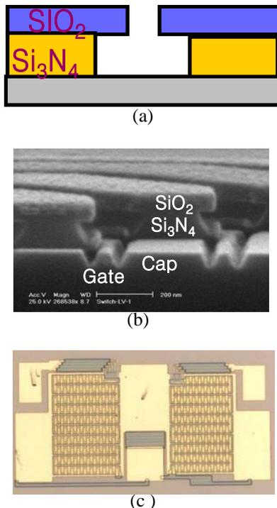
Fig. 1 (a) Schematic diagram of  $\text{SiO}_2/\text{Si}_3\text{N}_4$  dielectric overhang (b) SEM image of quadrate gate (c) top view of the fabricated SPDT switch
