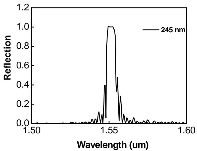
Fig 3. The simulation of the reflection for the DBR with period of 245 nm.
