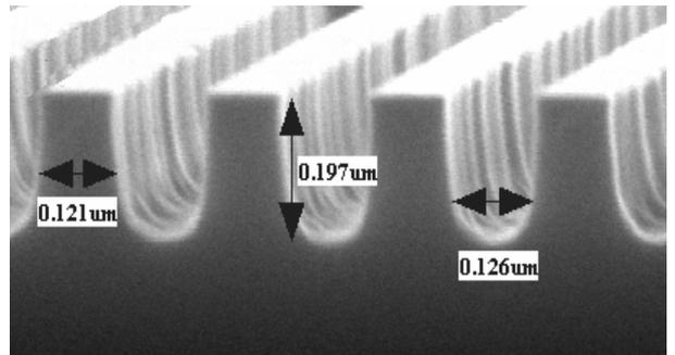
Fig 4. The SEM photograph of the DBR
