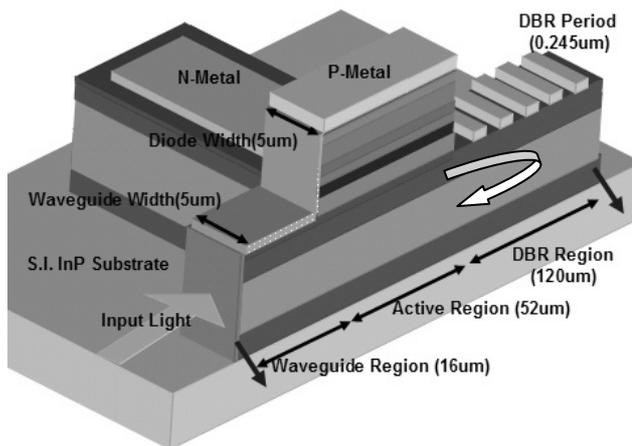
Fig 1. The cross-sectional view of the photodiode.
