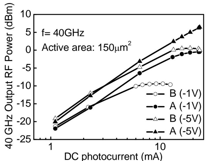
Fig 2. RF power versus dc photocurrent of device A and device B under different reverse bias voltages (close triangle: -5V of device A, open triangle: -5V of device B, close circle: -1V of device A, open circle: -1V of device B) at 40GHz operating frequency.
