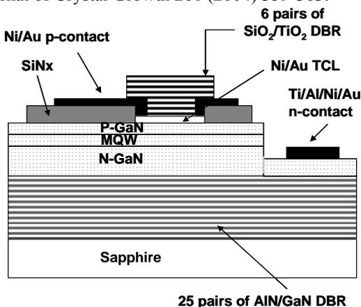
FIG1. Schematic of the GaN-based MCLED.
