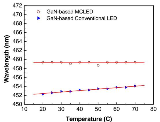
FIG6. EL of the GaN-based MCLED and the conventional LED as varying operating temperature at 1KA/cm<sup>2</sup> injection current density.
