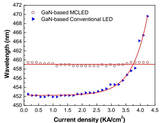
FIG5. EL of the GaN-based MCLED and the conventional LED as varying injection current density at 25°C.
