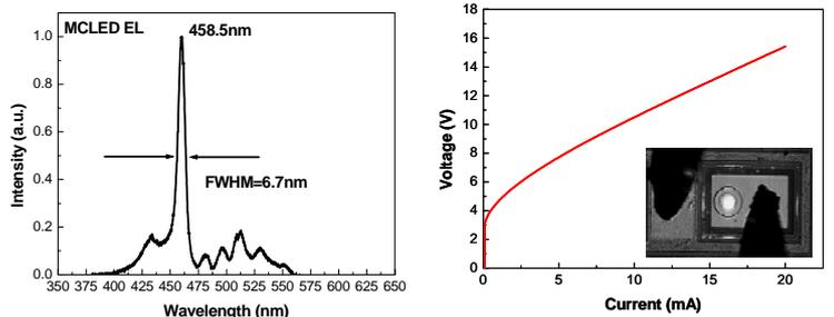
FIG3. Room temperature EL spectrum of the GaN-based MCLED with narrow FWHM of 6.7nm.
