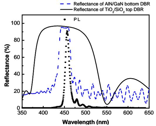
FIG2. Reflectance of 25 pairs of AlN/GaN bottom DBR and 6 pairs of TiO<sub>2</sub>/SiO<sub>2</sub> top DBR. The PL spectrum was also shown in the figure.
