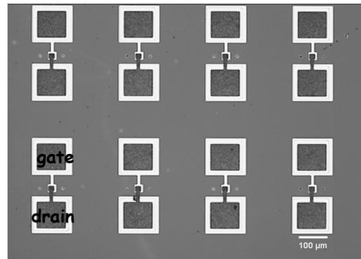
Fig 2 Airbridge (top) and device layout (below) of the completed transistor.
