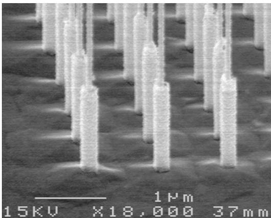
Fig. 1 Array of nanowires after gate formation.
