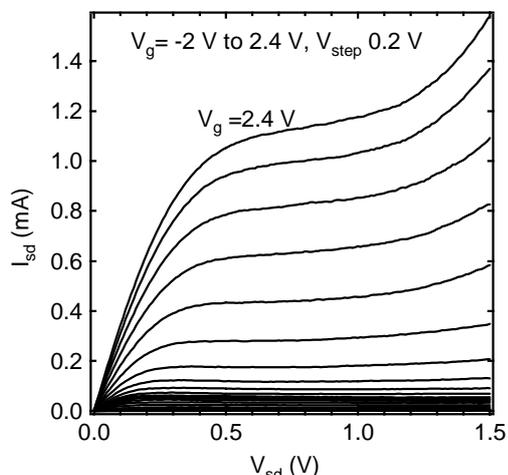
Fig 3 Room temperature characteristics of nanowire transistor consisting of 100 nanowires in parallel.
