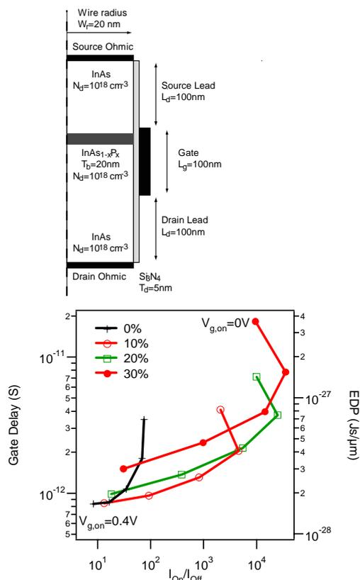
Fig 4 Simulated heterostructure nanowire FET. Design (above) and extracted data for different alloy compositions (P content) and gate voltages (below).
