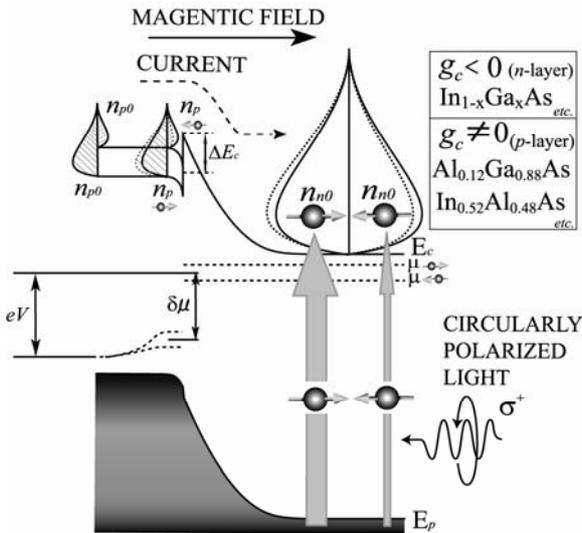
Fig.1 Schematic illustration showing the concept of the spin voltaic effect in a  $p$ - $n$  heterojunction with spin split in  $p$ -side. Circularly polarized light is illuminated on  $n$ -side.
