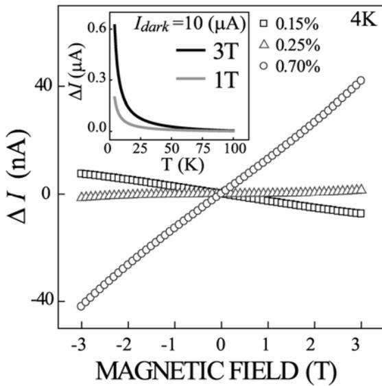
Fig2: Calculated  $\Delta I$ - $H$  curves at 4 K with three different  $P_n$  values. Inset shows temperature dependence of  $\Delta I$  with two different  $H$ .
