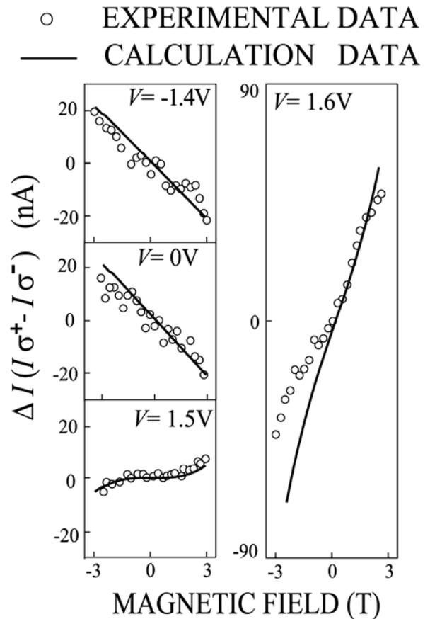
Fig3:  $\Delta I$  -  $H$  characteristics at 4 K with various bias voltage ( $V = -1.4, 0, 1.5, \text{ and } 1.6 \text{V}$ ).
