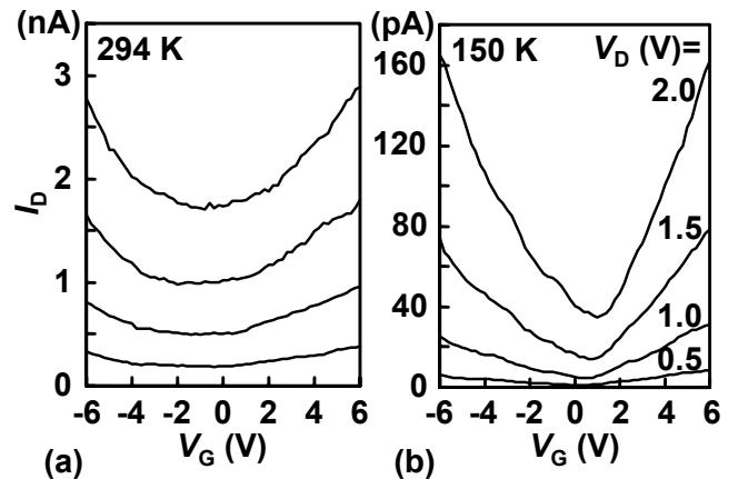
Fig. 6 Drain current-gate voltage characteristics for L=0.75 μm and W=1.0 μm at (a) 294 K and (b) 150 K, respectively. On-off current ratios of two and seven are attained, respectively.
