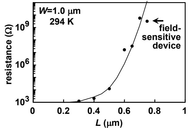
Fig. 5 Length dependence of the source-drain resistance of the devices with  $V_G=0$ . The resistance increases rapidly when the channel region is shadowed by the enlarged L (>0.5 μm). The devices with high resistance were found to be field-sensitive.
