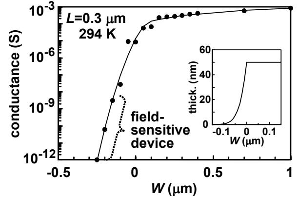
Fig. 4 Logarithmic plot of the same conductance as in Fig. 3, showing the feature of the tail part of the thickness distribution at the film edge. From the separate evaluation similar to Fig. 6, the devices with smaller conductance were found to be field-sensitive. Inset: Estimated thickness profile at the film edge.
