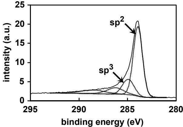
Fig. 2 C 1s XPS spectrum of the deposited carbon film. The sp<sup>2</sup> (graphite) component is dominant in the film. The small two peaks at higher energies are assigned to the C-O bond originated from the adsorbed oxygen [3].
