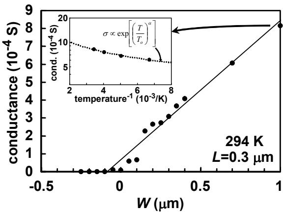
Fig. 3 Width dependence of the source-drain conductance of the devices with  $V_G=0$ . The slope of the fitted line is  $7.8 \times 10^{-4}$  S/μm. Inset: Temperature dependence of the conductance.
