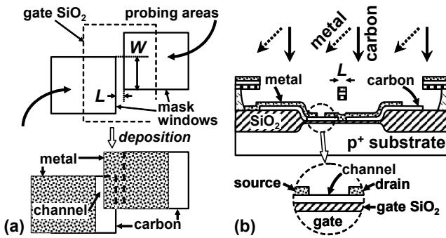
Fig. 1(a) Plane view of the deposition mask and deposited metal/carbon films, (b) cross-sectional view of the FET. Two-step process of vertical deposition of carbon and oblique (45°) deposition of metal finishes the FET without additional lithographic process.
