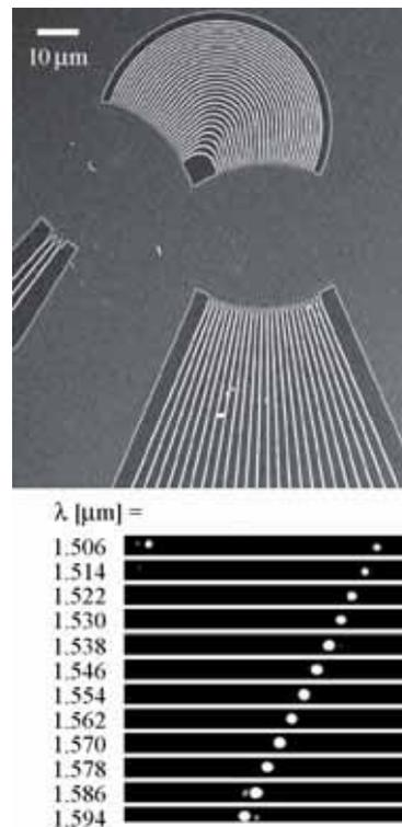
Fig. 5 Si wire AWG and output light.
