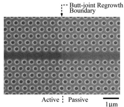
Fig. 2 Active/passive integrated PC slab laser.
