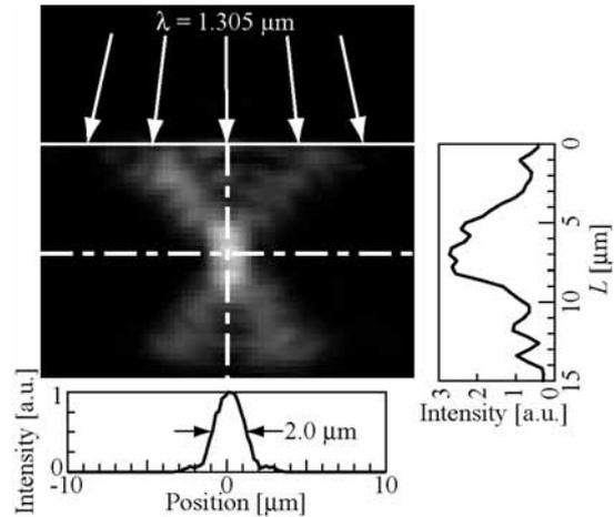
Fig. 4 Near field pattern of focused light in PC.
