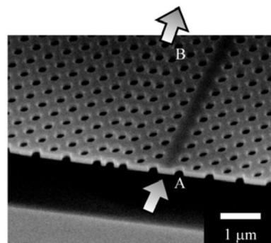
Fig. 3 PC directional coupler slow light device.
