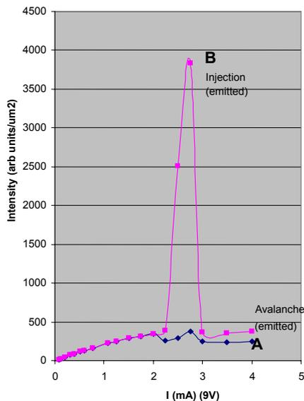
Fig. 4. Optical performance of the  $n^+$ pn bipolar like Si CMOS light emitting device with the main junction (site B) in avalanching reverse bias light emission mode and about 20% electron current injected into the junction.
