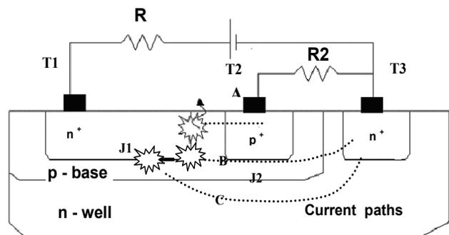
Fig. 1. Circuit and bias configuration for various modes of operation of a two junction BJT Si Light Emitting Device (LED) fabricated with Si CMOS technology. The origin of the light emission processes is schematically illustrated for current paths A, B and C, respectively.
