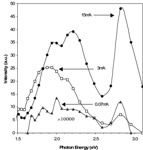
Fig. 5 Light emission intensity profiles for single junction (Site A) and two junction mode (Site B) light emission mode of operation (as were obtained for a second similarly designed device).
