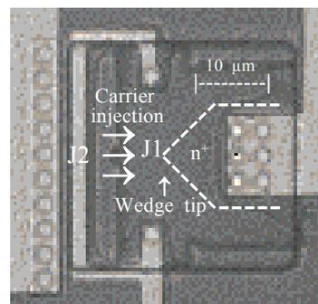
Fig. 2 Bright field optical micrograph showing the top surface of the device as well as the current configuration for current path C of operation with J2 injecting electrons into the avalanching junction J1.
