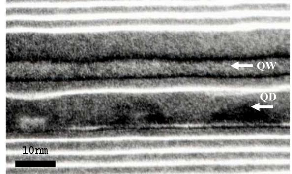
Fig. 2 TEM (200) dark-field micrographs of tunnel QW-on-QDs structure: 3 nm-thick  $\text{In}_{0.33}\text{Ga}_{0.67}\text{As}$  QW separated from the top of InAs QDs by a 4.5 nm-thick GaAs and AlAs (2ML) barrier.
