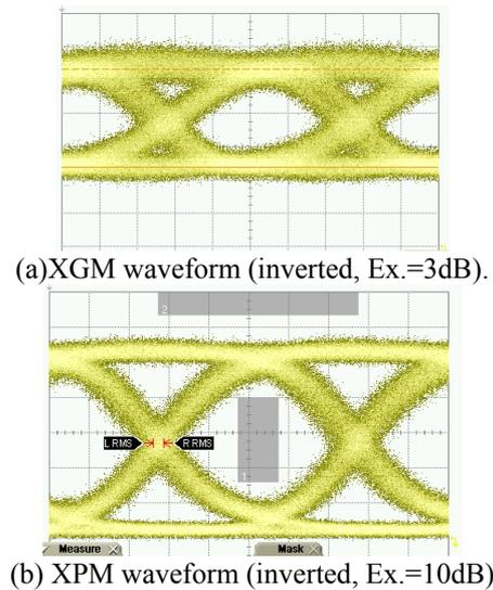
Fig. 7 Measured XGM and XPM waveform for 40G bit/s.
