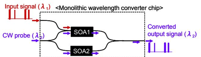
Fig. 2 Top view of the monolithic chip.
