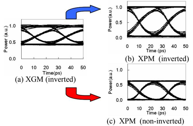
Fig. 6 Calculated waveform for XGM and XPM operation.
