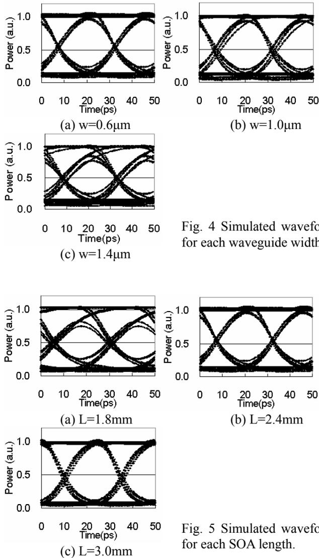
Fig. 4 Simulated waveform for each waveguide width.
