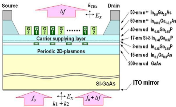
Fig. 1 Device structure used in our experiment with  $L_{G1} = 70$  nm and  $L_{G2} = 350$  nm.
