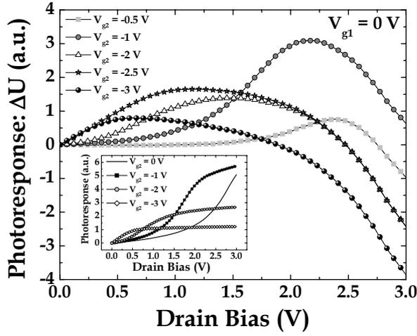
Fig. 2: Relative photoresponse vs.  $V_{ds}$  at  $V_{g1} = 0V$  for different  $V_{g2}$  values. Inset shows the photoresponse at  $V_{g1} = 0V$  and  $V_{g2} = -3 \sim 0 V$ .
