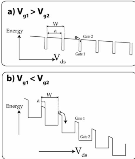
Fig. 3: Band diagrams for the case when: a)  $V_{g1} > V_{g2}$  and b)  $V_{g1} < V_{g2}$ .
