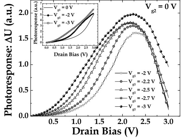
Fig. 4: Relative photoresponse vs.  $V_{ds}$  at  $V_{g2} = 0V$  for different  $V_{g1}$  values. Inset shows the photoresponse at  $V_{g2} = 0V$  and  $V_{g1} = -3 \sim 0 V$ .
