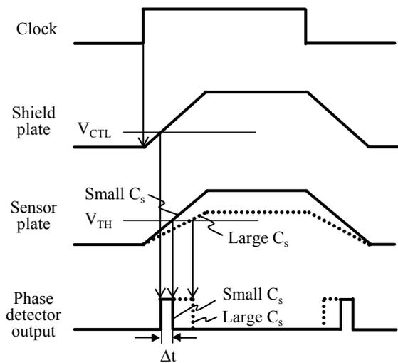
Fig. 3. Sensing circuit operation.
