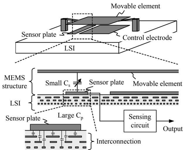
Fig. 1. MEMS variable capacitor stacked on LSI using capacitive-sensing to control the movable element.
