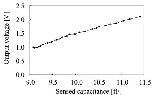
Fig. 6. Sensed capacitance vs. sensing circuit output (measured).
