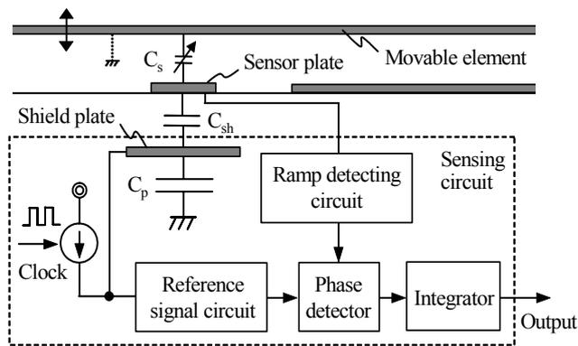
Fig. 2. Architecture for the proposed capacitive-sensing scheme.
