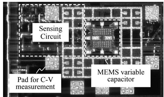
Fig. 5. Microphotograph of the test chip with the MEMS variable capacitor.
