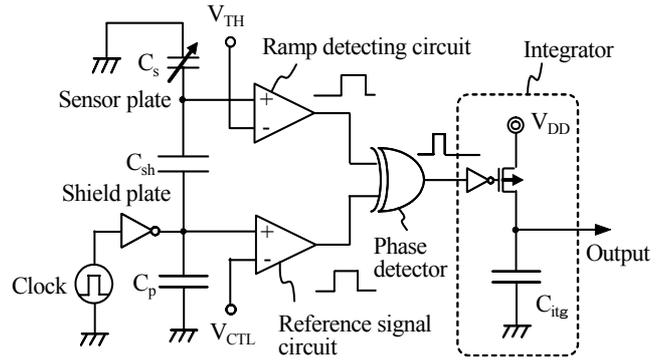
Fig. 4. Configuration of sensing circuit.
