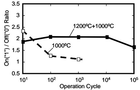
Fig. 7. Dependency of “on” to “off” current ratio on the writing cycle obtained from the  $\text{SiO}_x/\beta\text{-SiC/Si}$  resistive memory devices formed by one-stage oxidation and the two-stage oxidation process.
