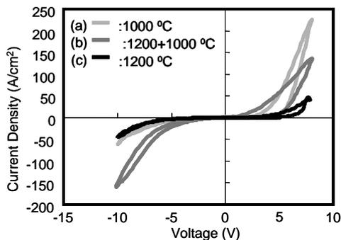
Fig. 6. Typical  $I$ - $V$  curves of the memory devices formed by oxidation (a) at  $1000^\circ\text{C}$ , (b) at  $1200^\circ\text{C}$  and then  $1000^\circ\text{C}$ , (c) at  $1200^\circ\text{C}$ .
