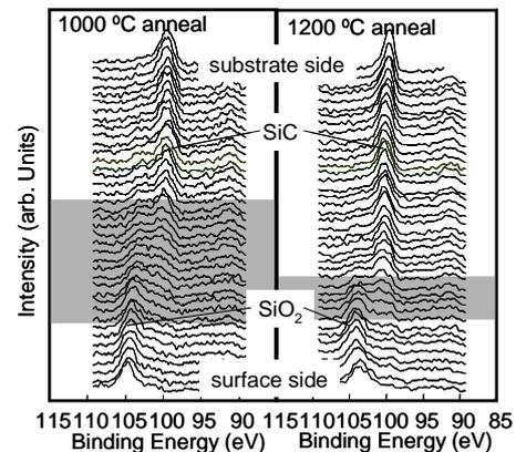
Fig. 3. XPS spectra obtained in the depth direction from SiC layers oxidized at 1000 °C and 1200 °C. The gray zones correspond to the imperfect Si oxide interfaces.
