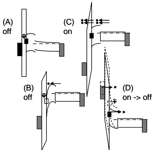
Fig. 4. The suggested memory function mechanisms of the  $\text{SiO}_x/\beta\text{-SiC/Si}$  resistive memory device.
