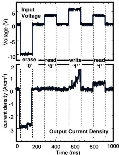
Fig. 5. Typical results of memory function. Input voltages and response currents are shown in the upper and lower figures, respectively.
