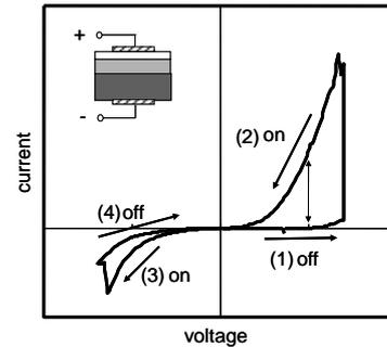
Fig. 2. A typical *I-V* curve of a SiO<sub>x</sub>/β-SiC/Si resistive memory device formed by one-stage oxidation at 1000 °C.
