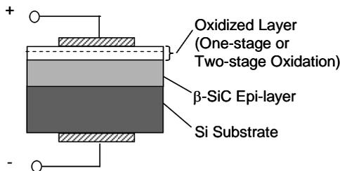
Fig. 1. The layer structure of the SiO<sub>x</sub>/β-SiC/Si resistive memory device. The oxide layer was formed by one-stage oxidation or the two-stage oxidation process (see text).
