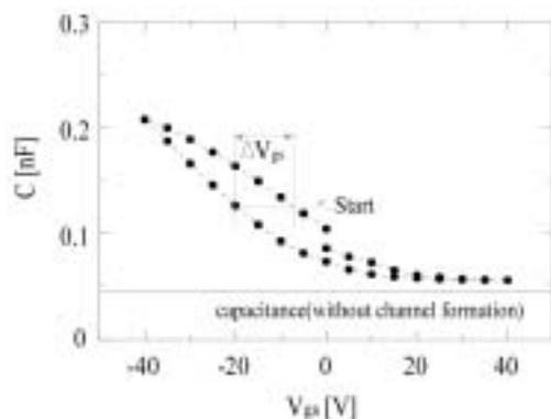
Fig. 1 The C-V measurement obtained for 100 nm pentacene FET using UV/ozone-OTS treated substrate
