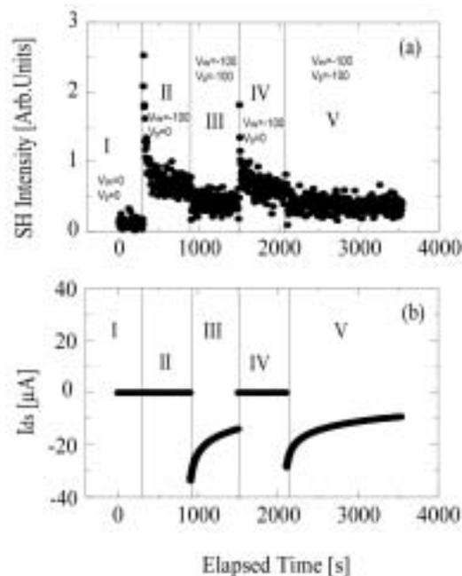
Fig. 2 Response of (a) the SHG with applying bias voltages and (b) the  $I_{ds}$  vs elapsed time for pentacene FET using UV/ozone-OTS treated substrate. Applied sequences are as follows; Region I ( $V_{ds}=0$ V,  $V_g=0$ V for 5 min.):Region II ( $V_{ds}=-100$ V,  $V_g=0$ V for 10 min.):Region III ( $V_{ds}=-100$ V,  $V_g=-100$ V for 10 min.):Region IV ( $V_{ds}=-100$ V,  $V_g=0$ V for 10 min.):Region V ( $V_{ds}=-100$ V,  $V_g=-100$ V for 20 min.)
