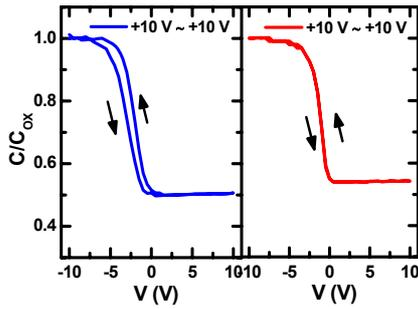
Fig. 3 Hysteresis of loop direction for HMDS- (left) PMMA (right) treated device.
