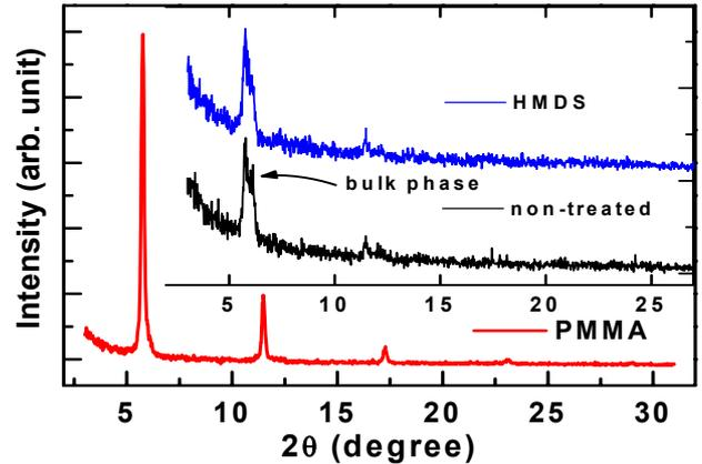
Fig. 4 XRD spectra of pentacene films with thickness of 50 nm at a substrate temperature of 70 °C for non-treated, HMDS and PMMA surface treated samples.
