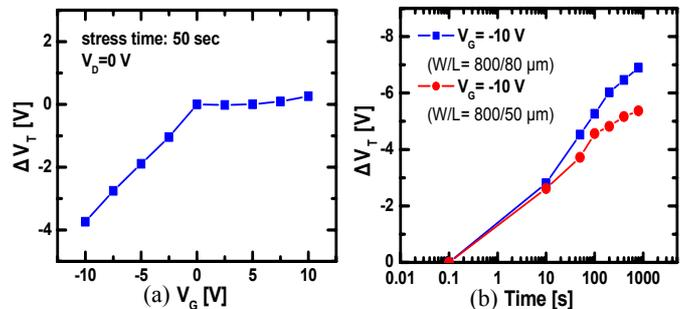
Fig. 2(a) Gate voltage dependence of threshold voltage shift under a fixed stressing time of 50 sec (b) Threshold voltage shift for transistors (W/L=800/80 μm and W/L=800/50 μm) as a function of time at a fixed gate bias of  $V_G=-10$  V.
