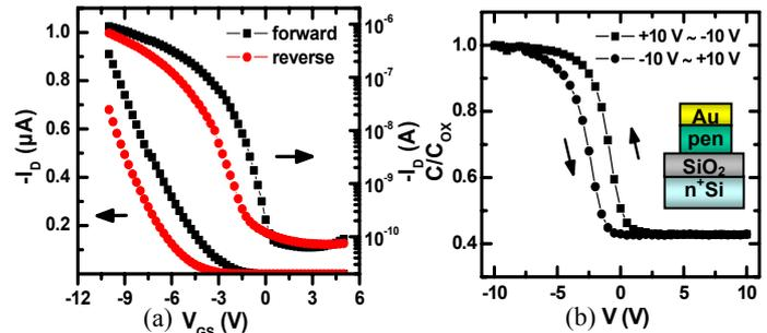
Fig. 1(a) Threshold voltage shift under bi-directional gate sweep: forward (+5 V → -10 V) and reverse (-10 V → +5 V) (b) Hysteresis of loop direction for bi-directional voltage sweep.
