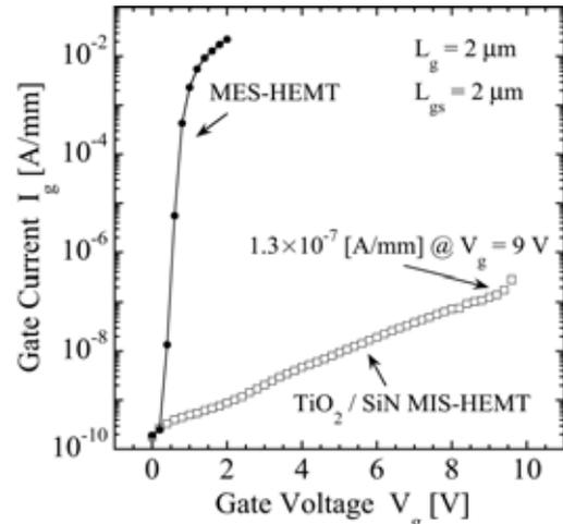
Fig. 2.  $I_g$ - $V_g$  characteristics of gate.
