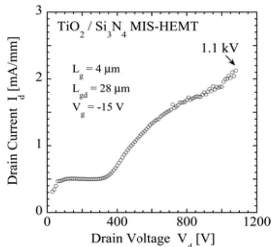
Fig.4. Off-state breakdown voltage behavior.
