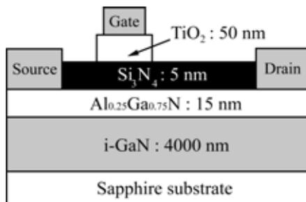
Fig.1. Schematic cross section of AlGaIn/GaN HEMT structure.
