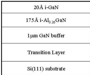
Fig. 1 Schematic of AlGaIn/GaN HEMT epi structure
