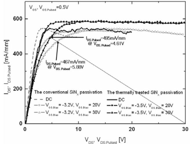
Fig. 4 Pulsed IV characteristics
