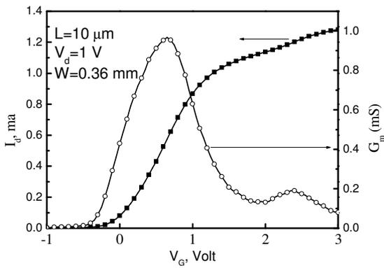
Figure 3.  $I_d$ - $V_g$  and  $g_m$ - $V_g$  characteristics of GaAs MOSFET with  $L/W=0.14$ .
