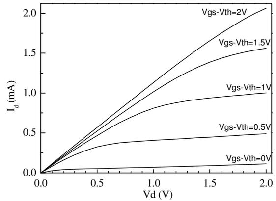
Figure 4.  $I_d$ - $V_d$  characteristics of GaAs MOSFET with  $L/W=0.14$ .
