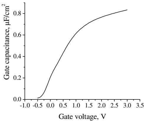
Figure 5. Gate-to-channel C-V characteristics of GaAs MOSFET
