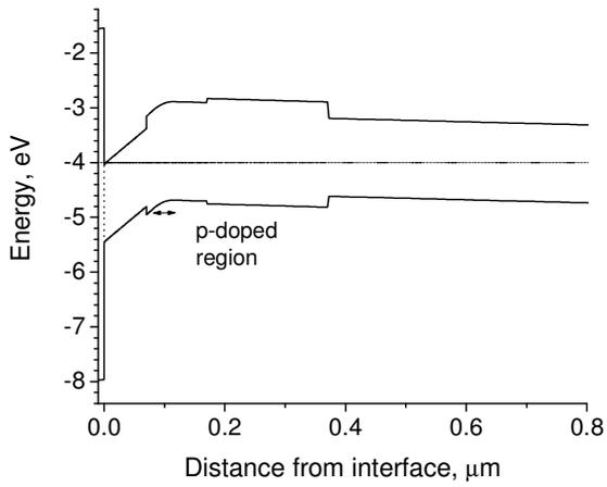
Figure 1 Band diagram of GaAs MOSFET in ON state (positive voltage applied to gate)
