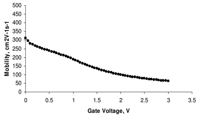
Figure 6. Effective electron mobility as a function of gate voltage on GaAs MOSFET
