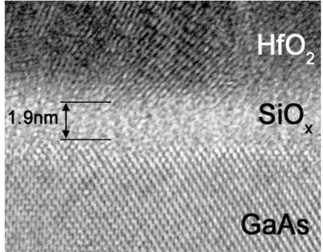
Figure 2 High resolution cross-sectional TEM of GaAs/SiO<sub>x</sub>/HfO<sub>2</sub> interface.
