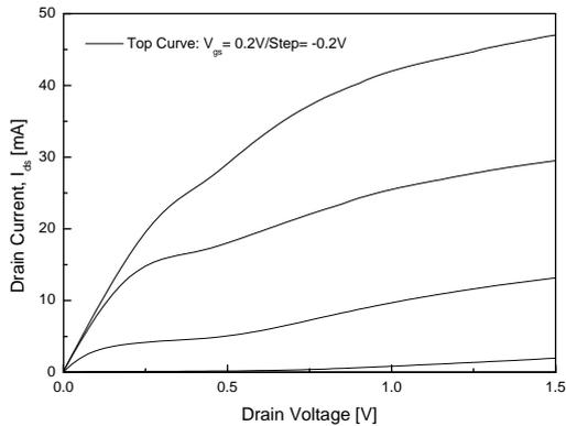
Fig. 3. I-V characteristics for 80nm T-gate MHEMTs.
