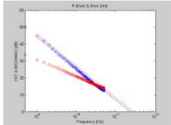
Fig. 5. Typical current gain,  $h_{21}$ , and MSG/MAG as a function of frequency for 80nm x 100  $\mu$ m low noise MHEMTs.
