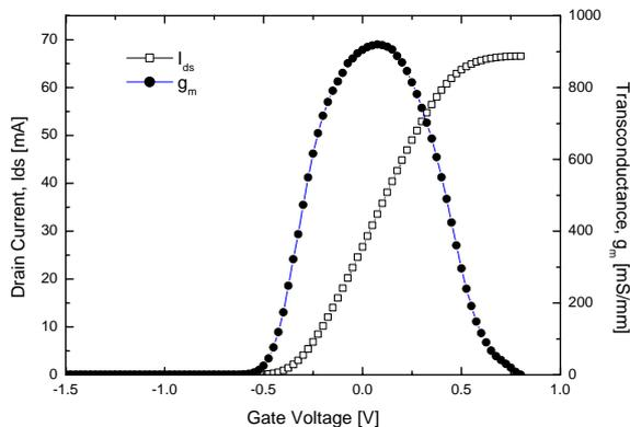
Fig. 4. Transfer characteristics for 80 nm x 100  $\mu$ m low noise MHEMTs.
