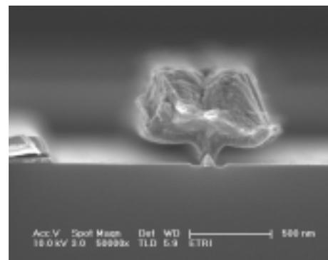
Fig. 2. Cross-sectional SEM of 80nm T-gate MHEMT with recess width of 50nm.
