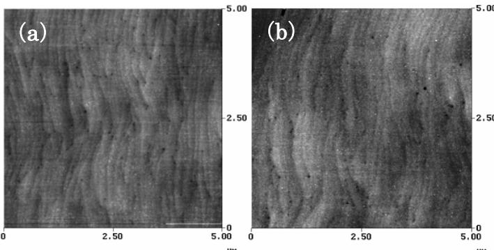
**Fig.2** AFM image of surfaces of GaN (a)before etching and (b)after etching for 30min with the etch-depth of about 38nm.
