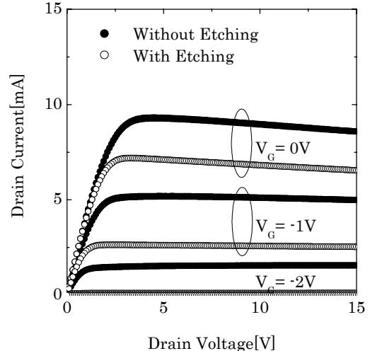
**Fig.4**  $I_D$ - $V_D$  characteristics of un-recessed and recessed gate HFETs. The gate length is  $2\mu\text{m}$  and width is  $50\mu\text{m}$ .
