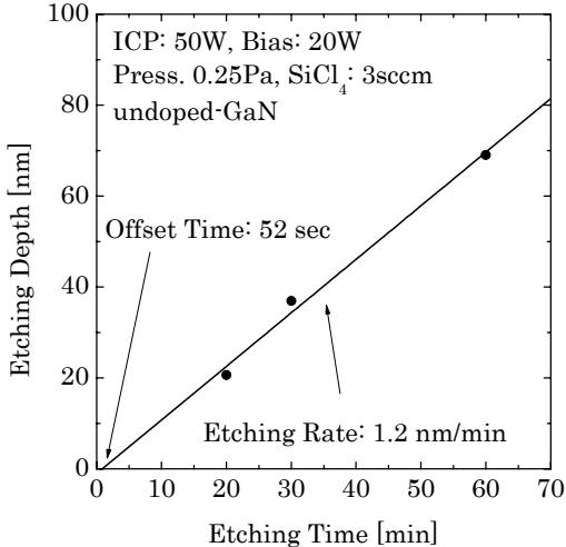
**Fig.1** Etching rate experiment on undoped GaN
