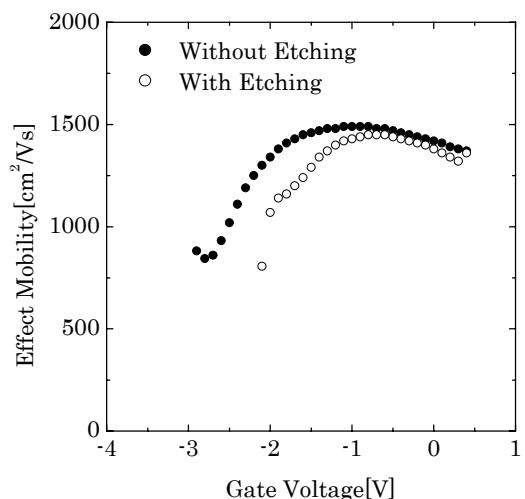
**Fig.6** Effective electron drift mobility for the FETs. Mobility was obtained from the ratio of  $I_D$  and the carrier concentration at the gate voltage. The carrier concentration was calculated by integration of the capacitance. The drain bias was 0.1V.
