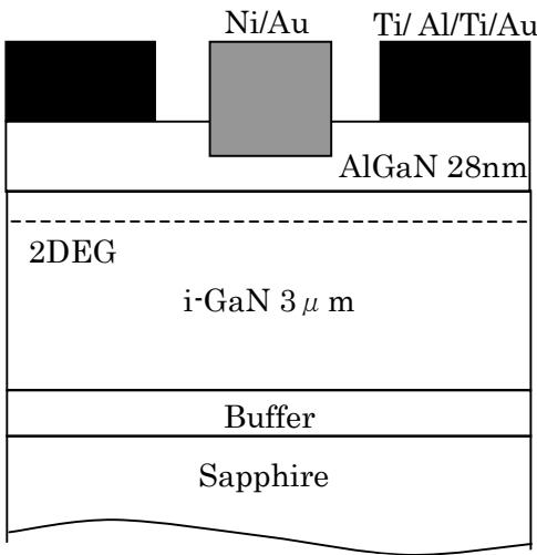
**Fig.3** Schematic cross-section of recessed gate AlGaN/GaN HFET.
