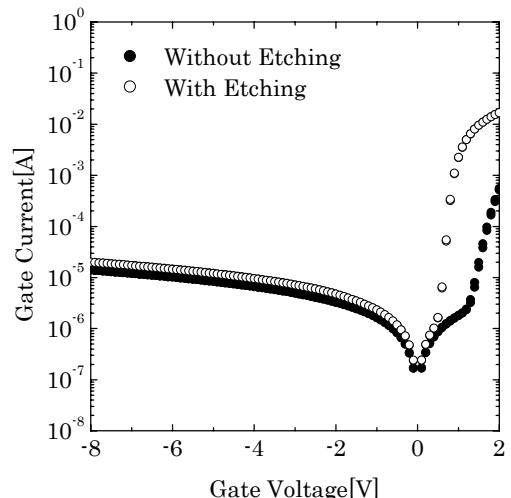
**Fig.5**  $I_G$ - $V_D$  characteristics of un-recessed and recessed gate HFETs. FET size is the same as those shown in Fig.4.
