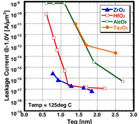
**Fig.3 Teq Dependence of Leakage Current @ 125 deg C**
