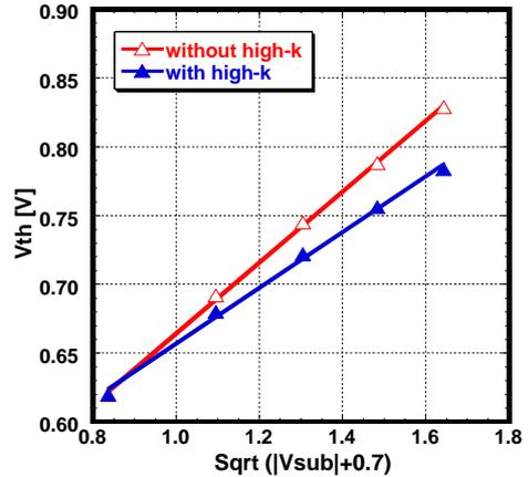
**Fig.5 Vth-Vsub of 55nm-node**
