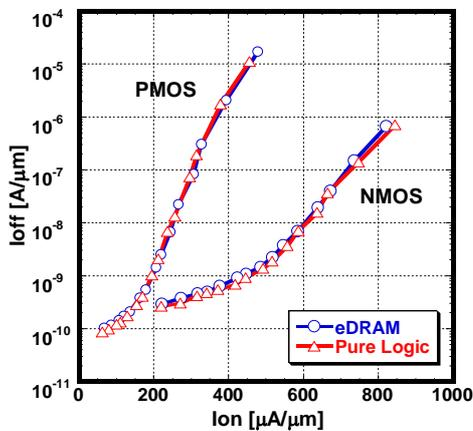
**Fig.4 Compatibility of Logic Trs. @ 90nm-node**
