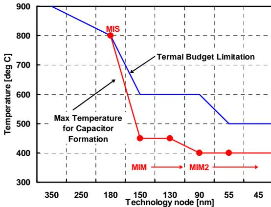
**Fig.2 Maximum Temperature for Capacitor Formation**
