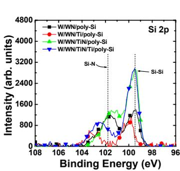
Fig. 4. XPS analysis for various gate stacks.
