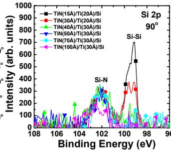
Fig. 2. XPS analysis for TiN/Ti diffusion barrier with various thicknesses.
