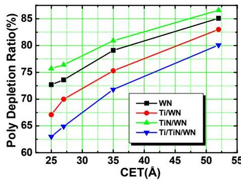
Fig. 9. Poly depletion ratio for different diffusion barriers.
