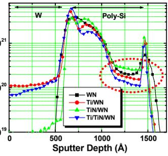
Fig. 7. Boron SIMS profiles for different gate stacks.
