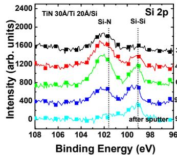
Fig. 1. XPS analysis for TiN/Ti diffusion barrier.
