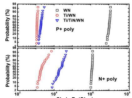
Fig. 13. Kelvin chain Rc for different barrier metals.
