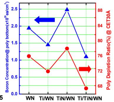
Fig. 10. Comparison between PDR and SIMS for different diffusion barriers.
