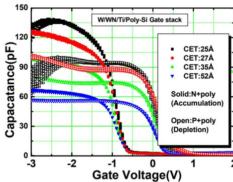
Fig. 8. Result of CV measurement for Ti/WN diffusion barrier.
