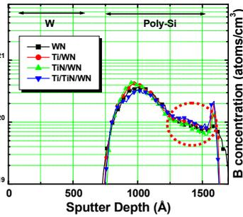
Fig. 6. Phosphorous SIMS profiles for different gate stacks.
