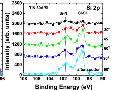
Fig. 3. XPS analysis for TiN diffusion barrier.
