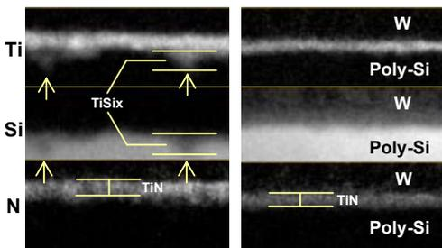
Fig. 11. EELS analysis for W/WN/Ti/Si gate stacks after post thermal treatment. Left (Ti:60Å), Right (Ti:30Å)
