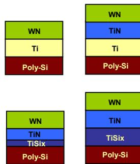
Fig. 12. Schematic cross section for W/WN/Ti/Si and W/WN/TiN/Ti/Si, Top ( As depo. ), Bottom ( After thermal process ).
