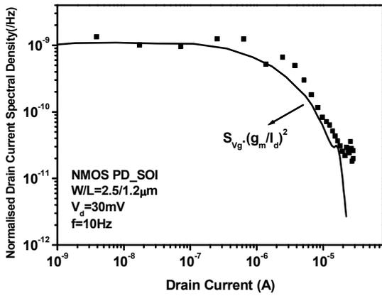
Fig. 1 Normalised drain current spectral density for a PD SOI with  $W/L=2.5/1.2\mu\text{m}$ , at  $V_d=30\text{mV}$  and  $f=10\text{Hz}$ .
