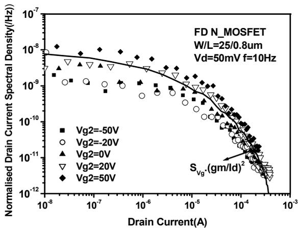
Fig. 3 Normalised drain current spectral density for a FD SOI with  $W/L=25/0.8\mu\text{m}$ , at  $V_d=50\text{mV}$ ,  $f=10\text{Hz}$  and  $V_{g2}=-50\dots50\text{V}$ .
