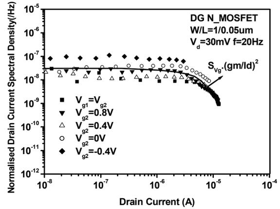
Fig. 5 Normalised drain current spectral density for a DG SOI with  $W/L=1/0.05\mu\text{m}$ , at  $V_d=30\text{mV}$ ,  $f=10\text{Hz}$  and  $V_{g2}=-0.4\dots0.8\text{V}$ .
