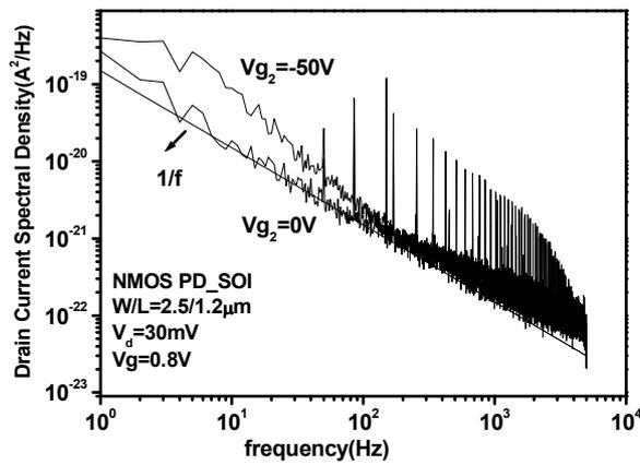
Fig. 2 Drain current spectral density for a PD SOI with  $W/L=2.5/1.2\mu\text{m}$ , at  $V_d=30\text{mV}$  and  $V_{g1}=0.8\text{V}$  for  $V_{g2}=0$  and  $-50\text{V}$ .
