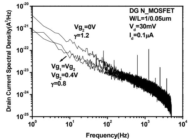
Fig. 6 Drain current spectral density for a DG SOI with  $W/L=1/0.05\mu\text{m}$ , at  $V_d=30\text{mV}$  and  $I_d=0.1\mu\text{A}$  for  $V_{g2}=0$  and  $0.4\text{V}$  and also  $V_{g1}=V_{g2}$  (double gate mode).
