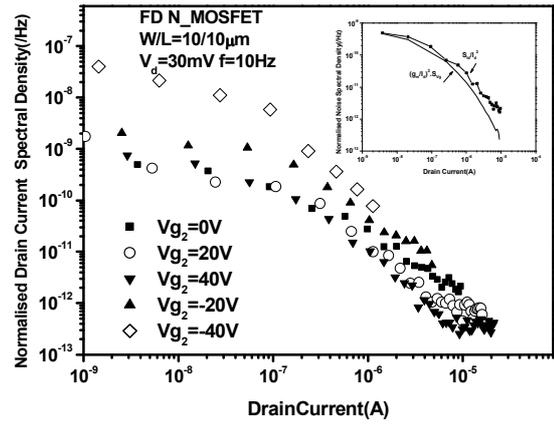
Fig. 4 Normalised drain current spectral density for a FD SOI with  $W/L=10/10\mu\text{m}$ , at  $V_d=30\text{mV}$ ,  $f=10\text{Hz}$  and  $V_{g2}=-40\dots40\text{V}$ .
