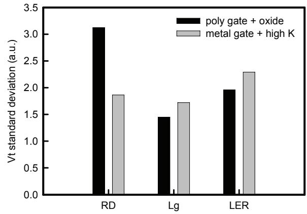
Figure 4. Normalized threshold voltage fluctuation components of poly-gate MOSFET and metal-gate and high- $\kappa$  materials MOSFET, where  $L_g$  is 25 nm and oxide thickness is 1.5 nm for the 32 nm technology node.
