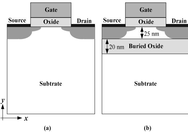
Figure 1. Cross-section views of the studied (a) planar MOSFET and (b) thin-buried-oxide SOI devices. Fluctuation of surface potentials for the explored device is computed in this study.
