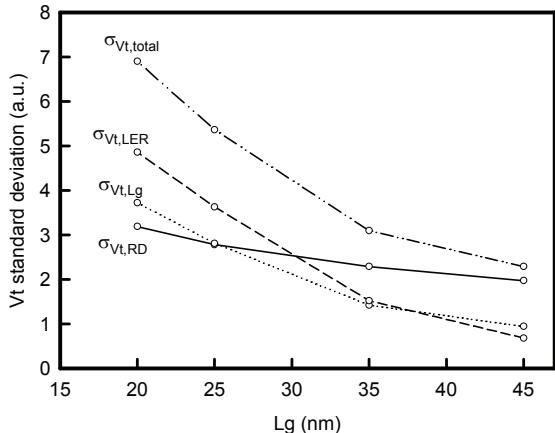
Figure 2. Normalized threshold voltage fluctuation of MOSFET devices. For 45 nm technology node, we assume that the nominal  $L_g$  of the device is 35 nm and oxide thickness is 1.7 nm. It includes  $\sigma_{vt, RD}$ ,  $\sigma_{vt,Lg}$  and  $\sigma_{vt,LER}$ , respectively.
