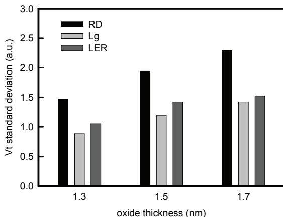
Figure 3. Normalized threshold voltage fluctuation versus the equivalent oxide thickness for a 35 nm MOSFET.
