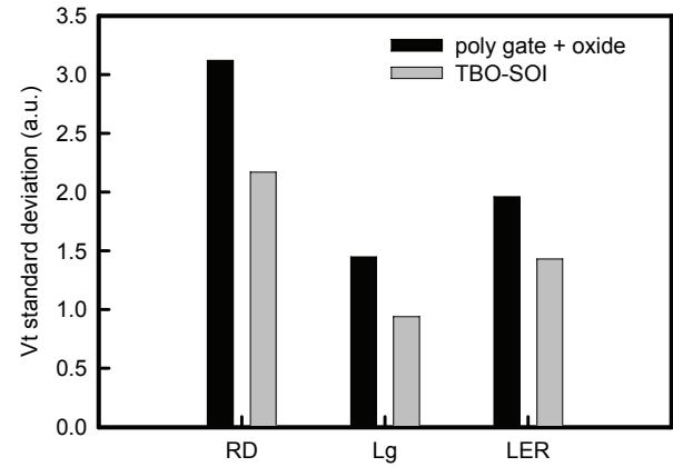
Figure 5. Normalized threshold voltage fluctuation components of poly-gate MOSFET and TBO SOI, where  $L_g$  is 25 nm and oxide thickness is 1.5 nm.
