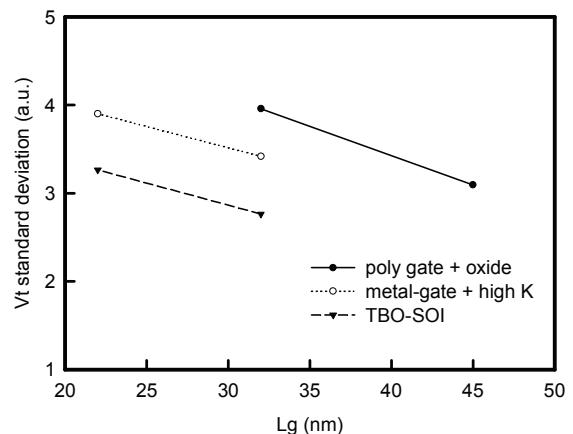
Figure 6. Normalized threshold voltage fluctuation versus the gate length for poly-gate, metal-gate + high- $\kappa$  MOSFETs, and thin-buried-oxide SOI.
