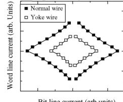
Fig.13 Asteroid curves with and without yoke wiring. 60% of the current can be reduced by the yoke.
