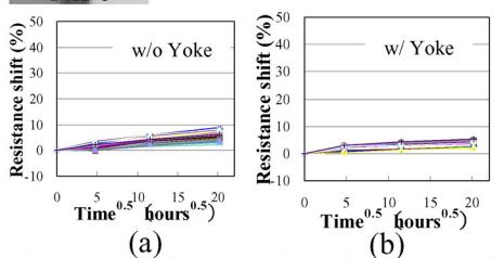
Fig.6 The stress induced void examination result of yoke wiring (a) and Cu wiring (b) respectively at 200 degree C. In yoke wiring, no resistance shift and good reliability results were obtained like Cu wiring.
