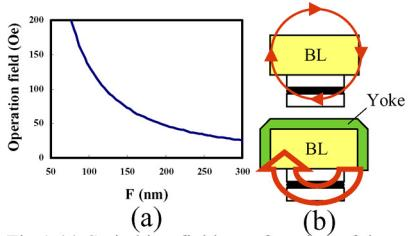
Fig.1 (a) Switching field as a function of the feature size. (b) Schematic illustrations of the magnetic field concentration effect of yoke
