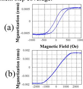
Fig.11 Magnetic hysteresis curves in the case of conventional sputtering (a) and high ionization sputtering (b). High ionization sputtering induces no remaining magnetic field .
