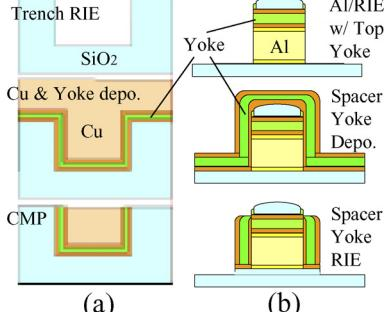
Fig.3 Process flow of our yoke wiring for a (a) word line and (b) bit line
