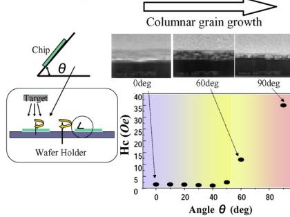
Fig.9 Grain growth and the switching field ( $H_c$ ) measured by a vibration sample magnetometer (VSM) for different sputtering angles of the conventional NiFe film.
