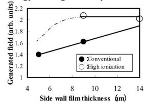
Fig.12 The ratio of current compares with the case of w/o yoke as a function of the sidewall film thickness in the case of high ionization sputtering and conventional sputtering respectively. The ratio of current increases by using high ionization sputtering.
