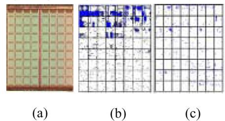
Fig.15 Photograph of the chip image of 16Mb MRAM (a). Failure bit maps of a 16Mbit without (b) and with the yoke wiring (c). By using the yoke wiring, the number of failing bits decreases drastically because of reduction in writing current.
