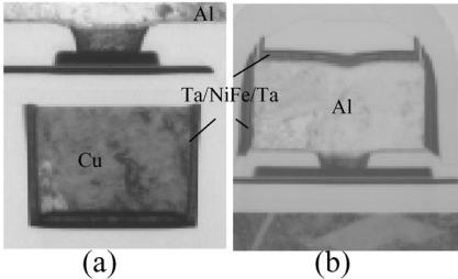
Fig.4 The cross-sectional TEM images of a (a) word line and (b) bit line with yoke.
