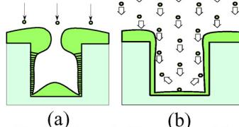
Fig.10 Schematic illustrations of the conventional process (a) and high ionization sputtering (b). High ionization sputtering suppresses columnar grain growth and realizes excellent step coverage.
