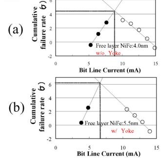
Fig.14 The effect of the yoke wiring on the writing margin. Sample (a) has a 4 nm thick free layer without yoke wiring. Sample (b) has a 5.5 nm thick free layer with yoke wiring. A closed circle stands for the selected state, that is, both WL and BL are selected. An open circle stands for a half-selected state, that is, only BL is selected. Sample (b) shows a large enough writing margin (more than  $6\sigma$ ).
