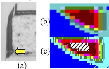
Fig.8 (a) The cross-sectional TEM image of a Bit line with a side-etched shape . The WL and BL current margin map are shown in (b) with the side-etched shape and in (c) after improving the side-etched shape. A hatched area of the map stands for no failures.
