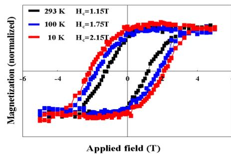
Figure 4. Temperature dependence of coercivity ( $H_c$ ) on the FePt nano-dots film annealed at 600°C for 1 hour measured by SQUID.
