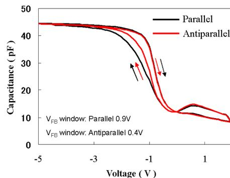
Figure 6. *C-V* characteristics of arrayed magnetic MOS capacitor.
