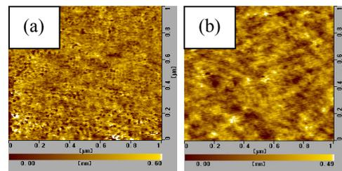
Figure 5. AFM result of FePt nano-dots film which formed on a silicon substrate with 10nm SiO<sub>2</sub> on its surface. (a) before and (b) after annealing at 600°C for 1 hour.
