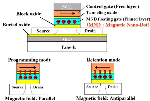
Figure 1. Cross-sectional structure and operating principle of MND memory.
