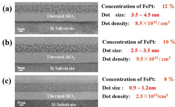
Figure 2. HRTEM cross-sectional images of 10-nm-thick FePt MND film formed on thermally oxidized silicon substrate: (a) FePt composition of 12%, (b) FePt composition of 10%, (c) FePt composition of 8%.
