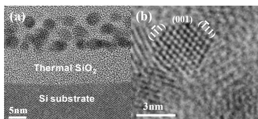
Figure 3. (a) HRTEM cross-sectional images of FePt MND film after annealing at 600°C for 1 hour. (b) Enlarged image of FePt nano-dot after annealing at 600°C for 1 hour.
