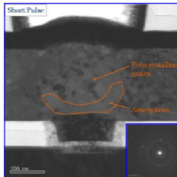
Fig. 7 TEM cross-sectional micrograph of PCM device programmed with a short SET pulse of 50 ns
