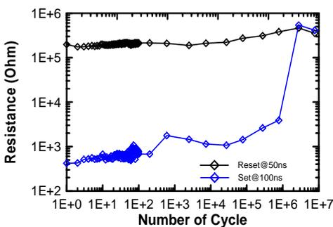
Fig. 9 Endurance performance of PCM device programmed with a short SET pulse of 100 ns
