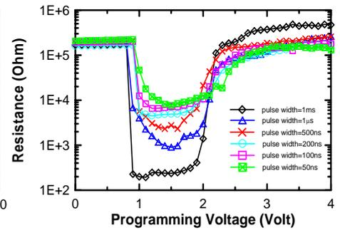
Fig. 5 Measured amorphous state R-V curves as a function of pulse width
