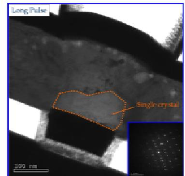
Fig. 8 TEM cross-sectional micrograph of PCM device programmed with a long SET pulse of 1 ms
