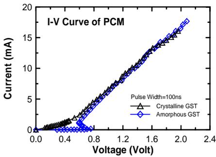
Fig. 3 Measured I-V curve of PCM device with the pulse width of 100 ns
