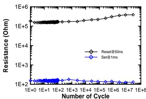
Fig. 10 Endurance performance of PCM device programmed with a long SET pulse of 1 ms
