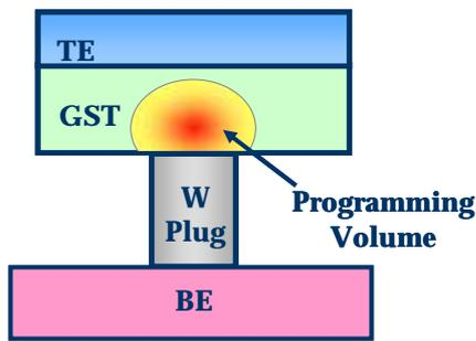
Fig. 1 Schematic cross section of PCM device with T-shaped structure
