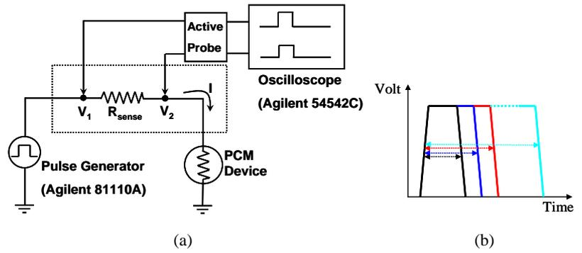
Fig. 2 Schematic view of (a) measurement setup and (b) programming strategy used to evaluate the PCM devices
