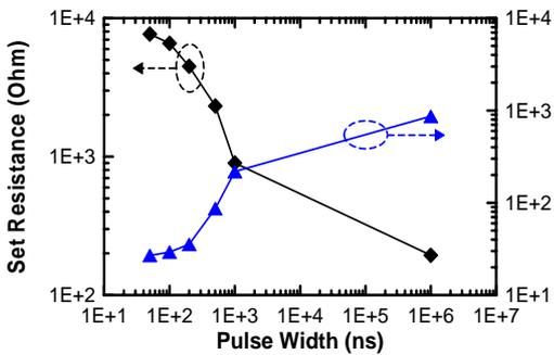
Fig. 6 Estimated SET resistance and sensing margin as a function of pulse width
