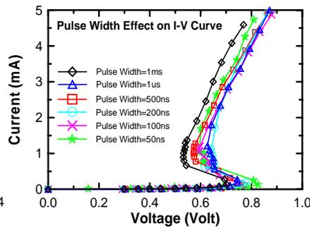
Fig. 4 Measured amorphous state I-V curves as a function of pulse width
