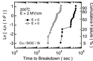
Fig. 5 *t*<sub>BD</sub> distribution of the blanket SiOC MIS capacitors.
