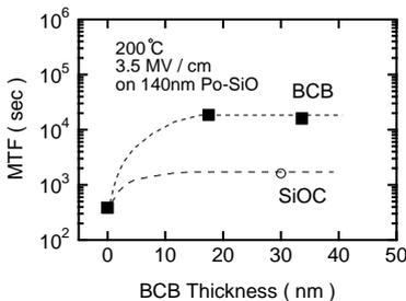
Fig. 7 MTF as a function of BCB or SiOC thickness.
