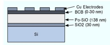
Fig. 3 Thin-BCB/porous silica (Po-SiO)/SiO<sub>2</sub> stacked MIS structure for electrical measurements.
