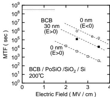
Fig. 8 Field dependent MTF for stacked MIS structures.
