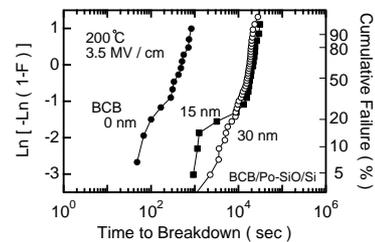
Fig. 6 *t*<sub>BD</sub> of the Cu/BCB/Po-SiO stacked MIS structures.
