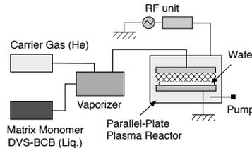
Fig. 2 Schematic diagram of a plasma-enhanced polymerization system.
