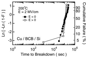
Fig. 4 Weibull plot of *t*<sub>BD</sub> for a blanket BCB film with Cu electrodes.
