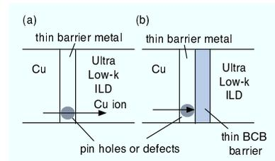
Fig. 9 Cu ion drift through a defect in thin barrier metal (a) and its suppression by forming a thin BCB barrier layer (b).
