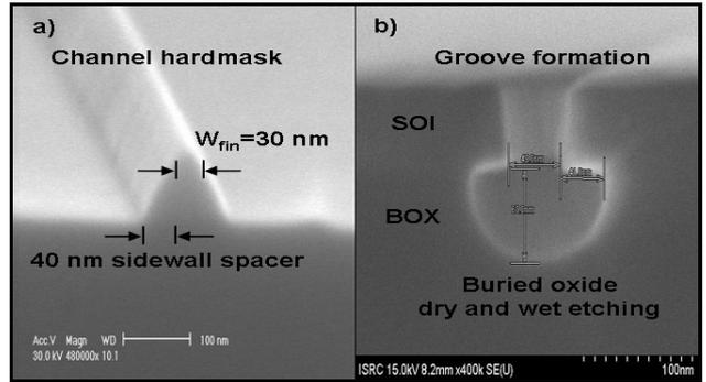
Fig. 3 SEM images of a) the channel hardmask and b) the groove region. Minimal groove width is 40 nm.
