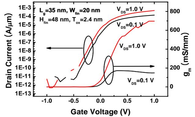
Fig. 4  $I_d$ - $V_g$  characteristics of a self-aligned GAA MOSFET. The gate length and the fin width are 35 and 20 nm, respectively.
