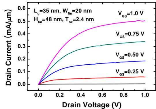
Fig. 5  $I_d$ - $V_d$  characteristics of the self-aligned GAA MOSFET. Due to the large source/drain structure, driving current is high.
