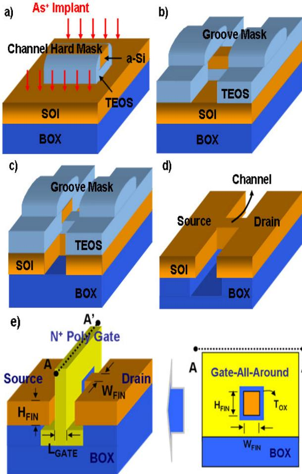
Fig. 1 Key process flow sequence and schematic diagram including the bird's eye view of the self-aligned GAA MOSFETs.
