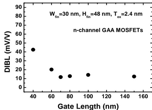
Fig. 6 DIBL as function of physical gate length for the fabricated self-aligned GAA MOSFETs.
