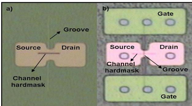
Fig. 2 Top view microscope images of the device a) after the groove formation and b) the photo-lithography for the contact.
