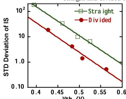
Fig. 4(b). Standard deviation of IS with respect to Vth.
