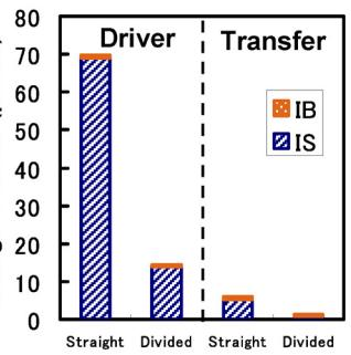
Fig. 3. Leakage components of driver and transfer transistors.
