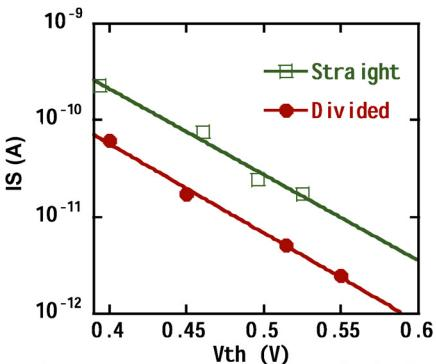
Fig. 8. IS current as a function of Vth of driver transistor.
