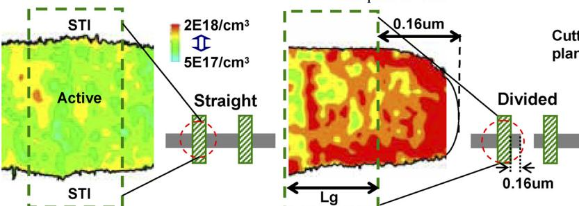
Fig. 6. STM images of p-type impurity (boron) on active field of driver transistors.
