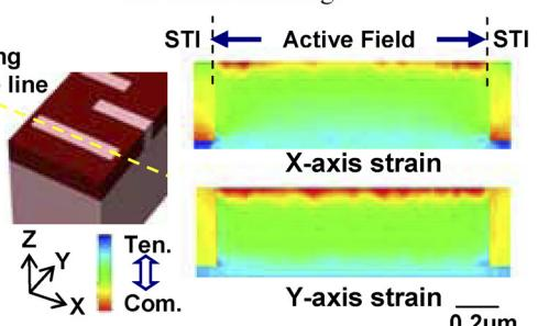
Fig. 7. 3-D simulated distribution of Si strain in direction of x- and y-axes around STI spacer during gate oxidation above 900°C.
