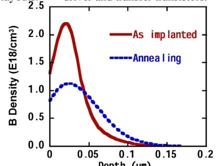
Fig. 5. Simulated B depth profile before and after Annealing.
