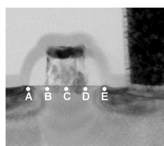
Fig. 9. Comparison of Si strain around driver gate electrode. Marks labeled with Roman letters in TEM image are strain measurement points.
