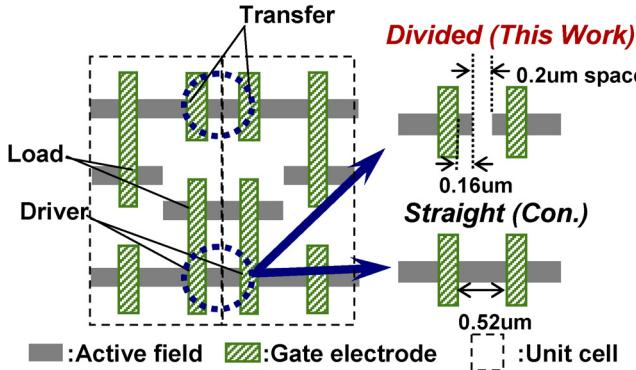
Fig. 1. Structure of the SRAM cell layouts examined in this work.
