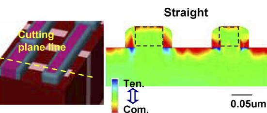
Fig. 10. 3-D-simulated Si strain distribution in direction of gate length for 45-nm node straight- and divided-type SRAM.
