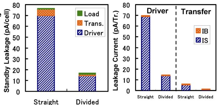
Fig. 2. Standby leakage current for straight and divided cell layouts.
