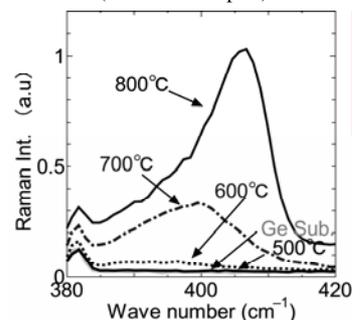
Fig. 10 Raman spectroscopy of fabricated devices with the Ge thickness of 16 nm in comparison with bulk Ge. The peak nearly  $400 \text{ cm}^{-1}$  indicates Si-Ge in SiGe.
