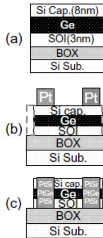
Fig. 3 The fabrication steps of proposed GOI MOSFET.
