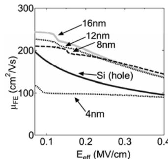
Fig. 8 The Ge thickness dependence of effective hole mobility of fabricated GOI pMOSFETs annealed at  $600 \text{ }^\circ\text{C}$  compared with the Si hole universal mobility.
