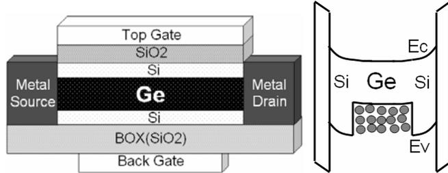
Fig. 1 Cross section of proposed device structure.
