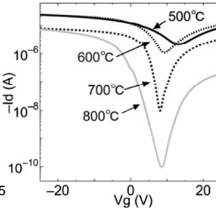
Fig. 6  $V_g$ - $I_d$  characteristics of GOI with the Ge thickness of 16 nm as a parameter of the annealing temperature. The Ion/off ratio increases with increasing the annealing temperature.
