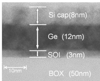
Fig. 4 Cross sectional TEM image of As-grown samples. (12nm-Ge samples)
