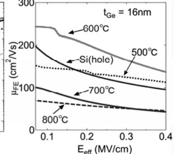
Fig. 7 The annealing temperature dependence of effective hole mobility of fabricated GOI pMOSFETs compared with the Si universal hole mobility. (16nm-Ge samples)
