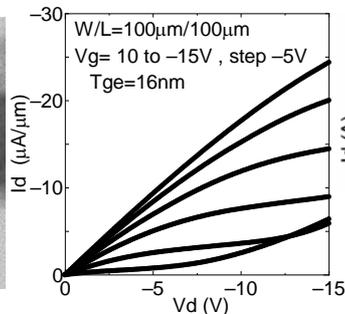
Fig. 5  $V_d$ - $I_d$  characteristics of fabricated GOI pMOSFETs. (16nm-Ge samples, annealing at  $600 \text{ }^\circ\text{C}$ )
