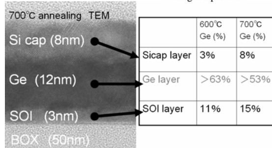
Fig. 9 Cross sectional TEM image of  $700 \text{ }^\circ\text{C}$  annealing samples with EDX. (12nm-Ge samples). The Ge concentration decreased with an increase in the annealing temperature.
