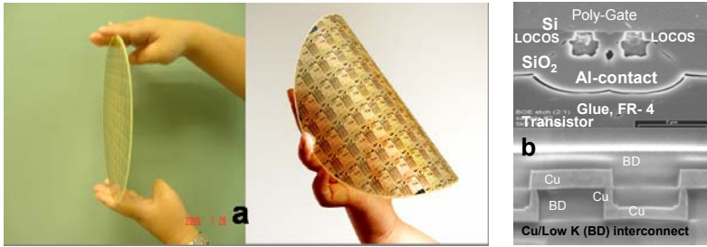
Fig.1. The devices on the FR-4 (4 mils) after WTT (a) The cross-section of transistor and Cu/Low K (BD) interconnect on flexible organic-substrate(FR-4) (b).
